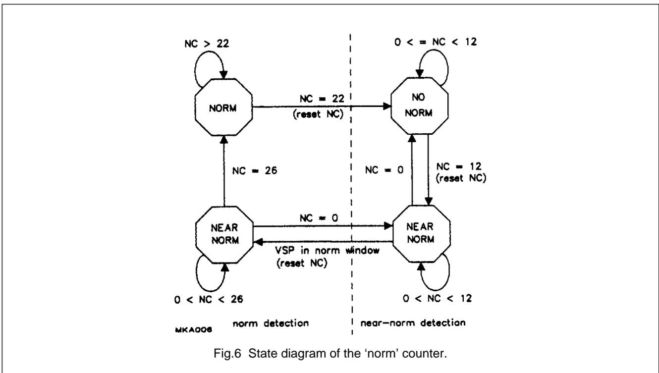
Fig.6 State diagram of the 'norm' counter.
