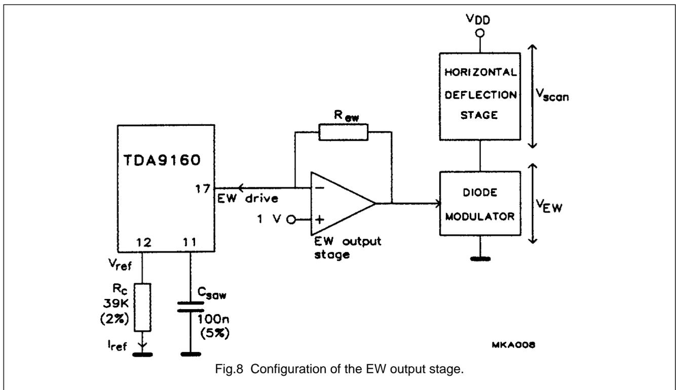
Fig.8 Configuration of the EW output stage.
