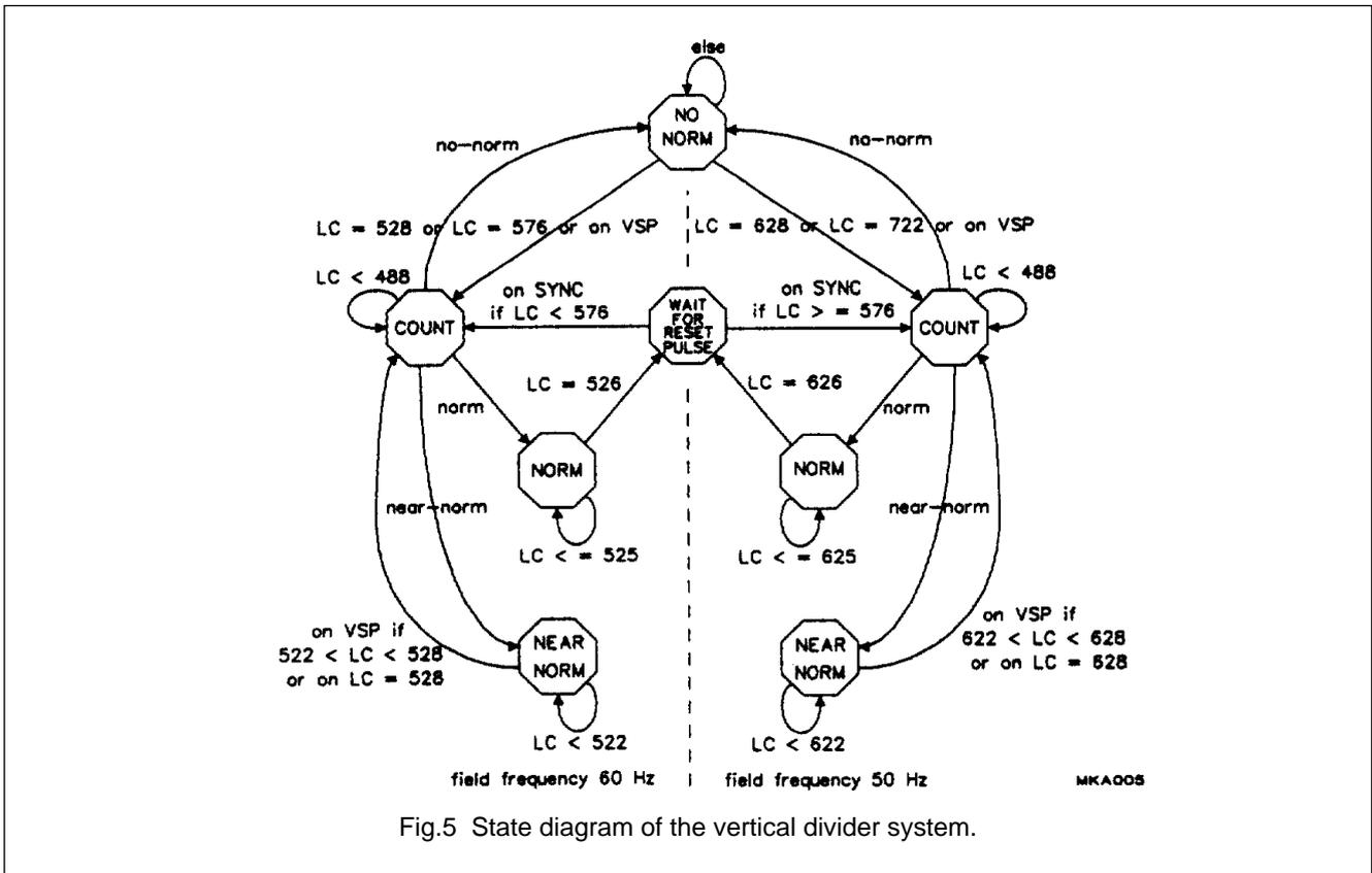
Fig.5 State diagram of the vertical divider system.
