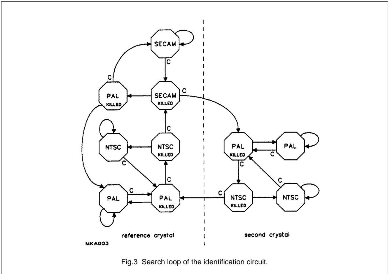
Fig.3 Search loop of the identification circuit.
