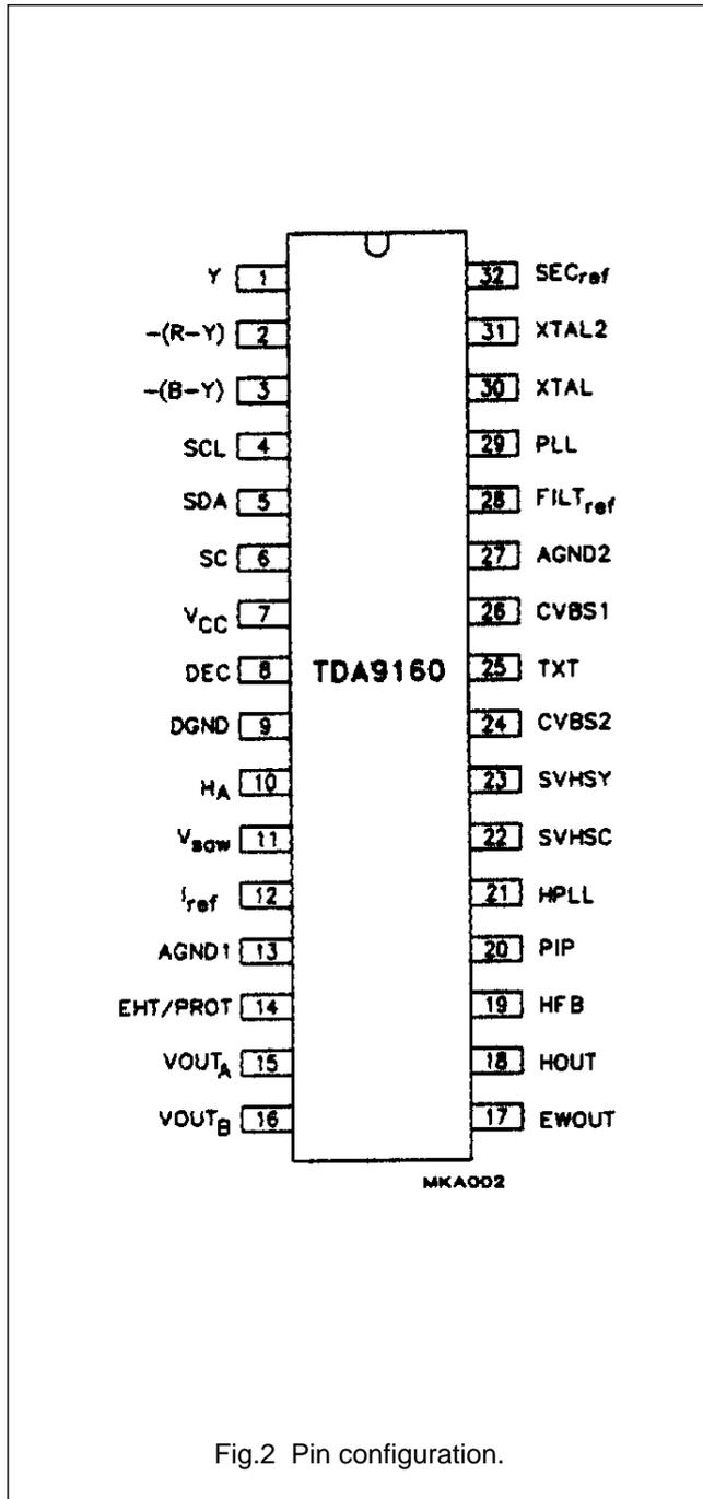
Fig.2 Pin configuration.
