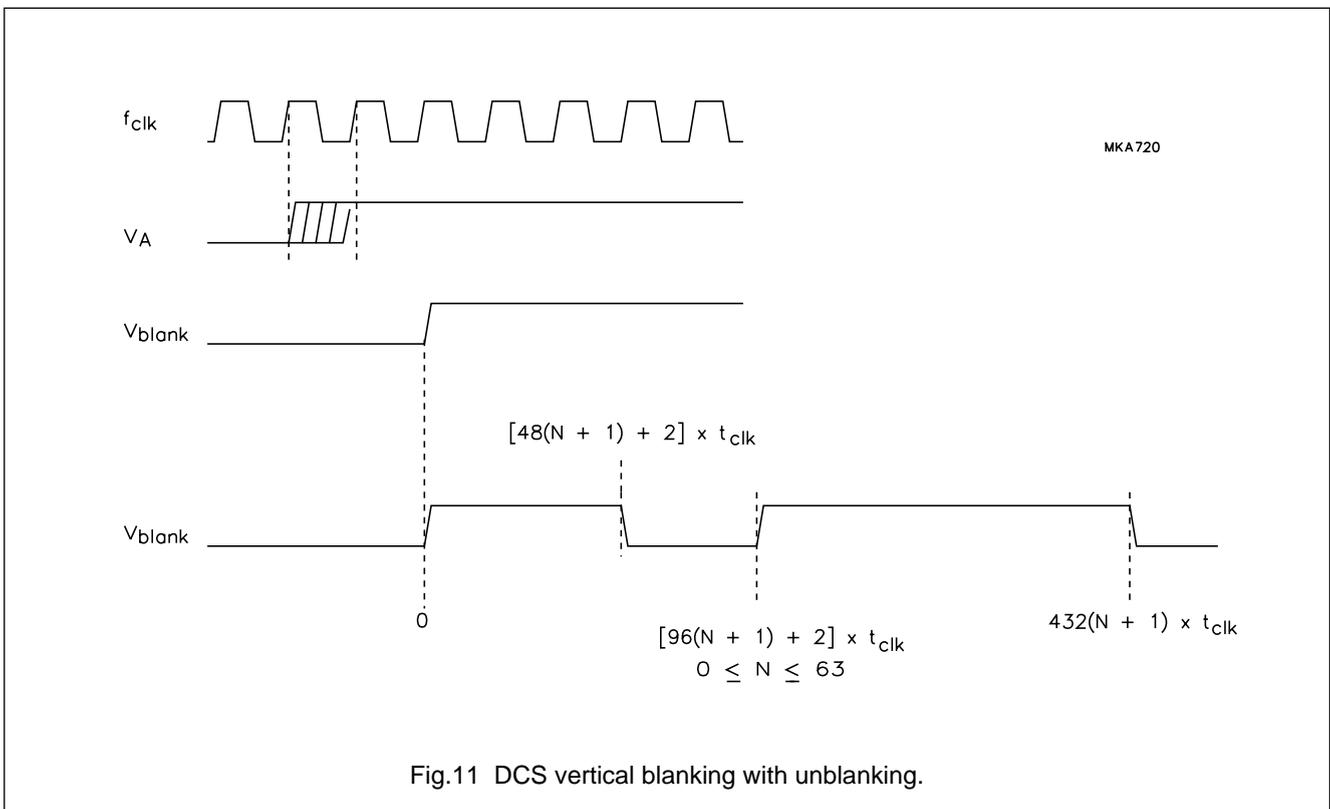
Fig.11 DCS vertical blanking with unblanking.
