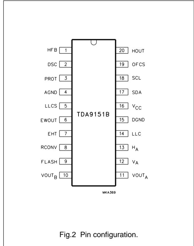
Fig.2 Pin configuration.
