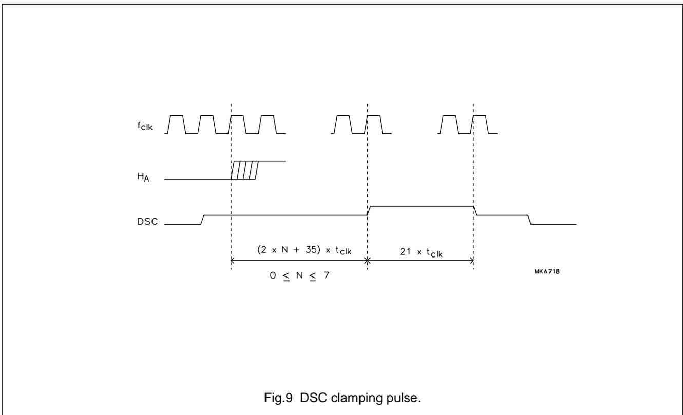
Fig.9 DSC clamping pulse.
