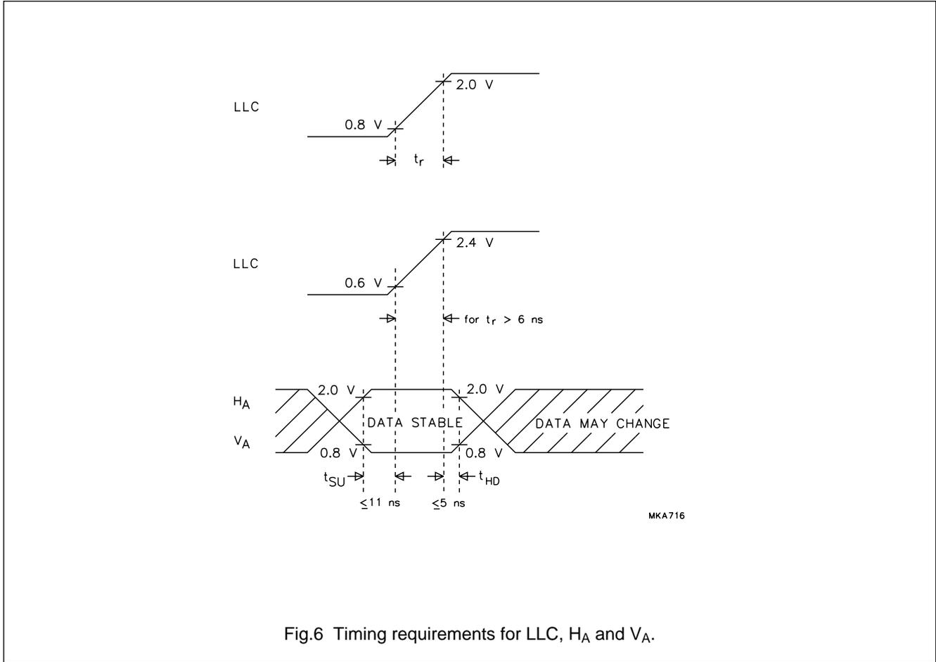
Fig.6 Timing requirements for LLC, HA and VA.
