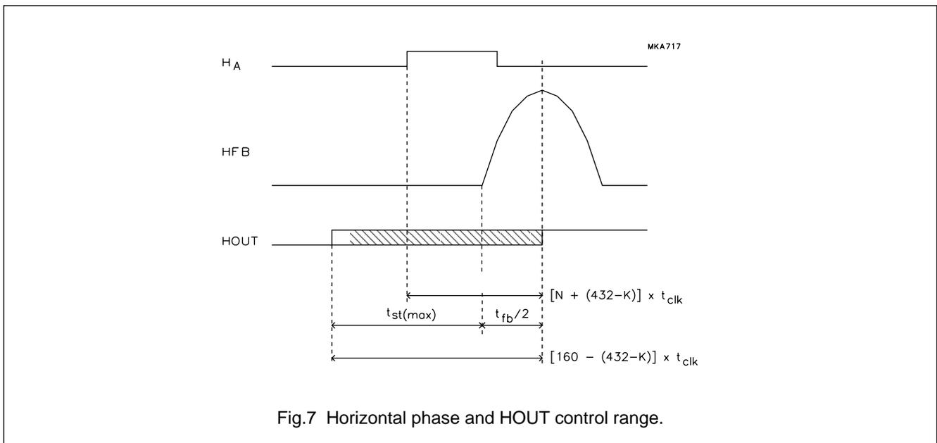
Fig.7 Horizontal phase and HOUT control range.
