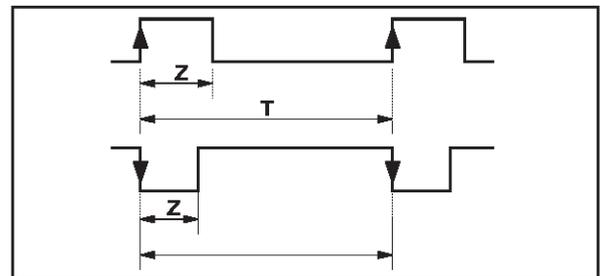
Using internal integration, both signals are recognized if  $Z/T < 25\%$ . Synchronization occurs on the leading edge of the internal sync signal. The minimum value of Z is 0.7 $\mu$ s.
