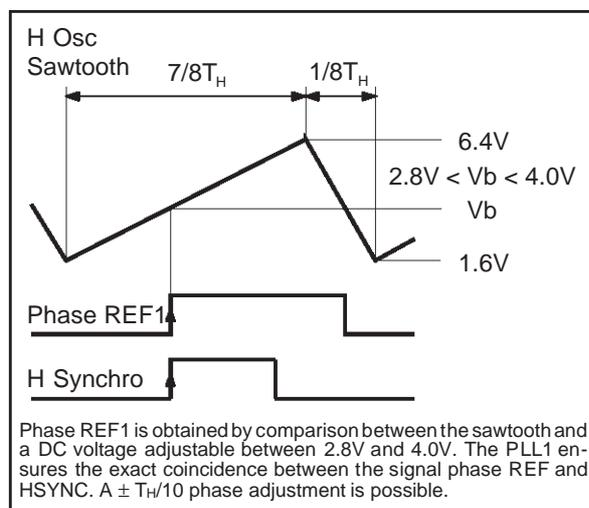
The TDA9109/SN also includes a Lock/Unlock identification block which senses in real time whether PLL1 is locked or not on the incoming horizontal sync signal. The resulting information is
