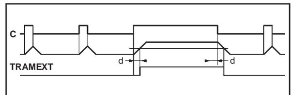
The last feature performed is the removal of equalization pulses to avoid parasitic pulses on the phase comparator (which would be disturbed by missing or extraneous pulses).
