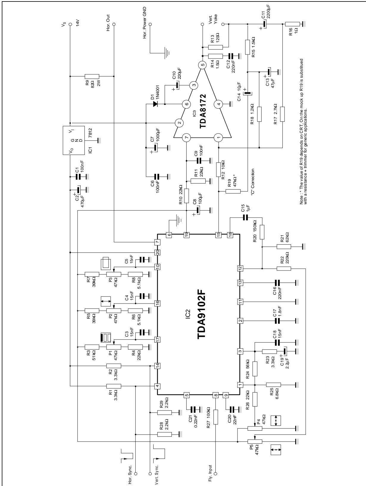
Note : \* The value of R19 depends on CRT. On the mock up R19 is substituted with a resistance + trimmer for generic applications.
