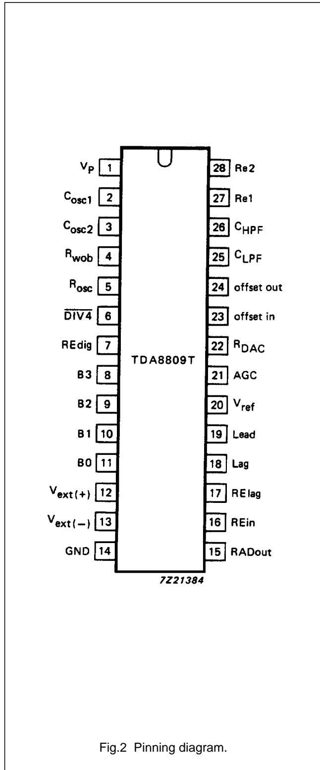
Fig.2 Pinning diagram.
