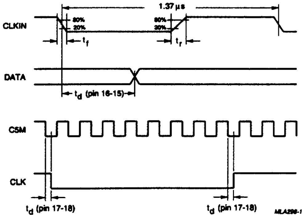
Fig.3 Data timing diagram.
