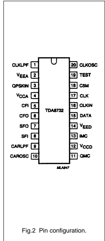
Fig.2 Pin configuration.
