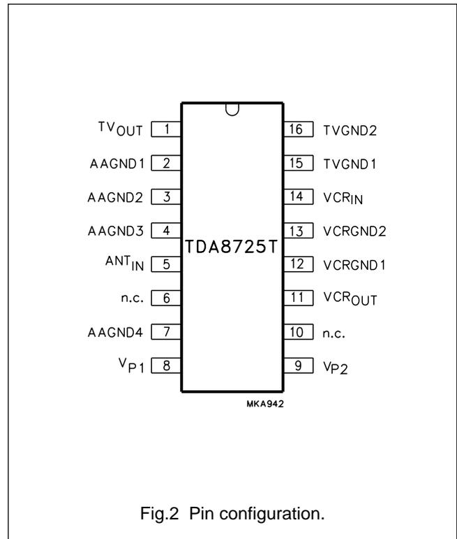
Fig.2 Pin configuration.
