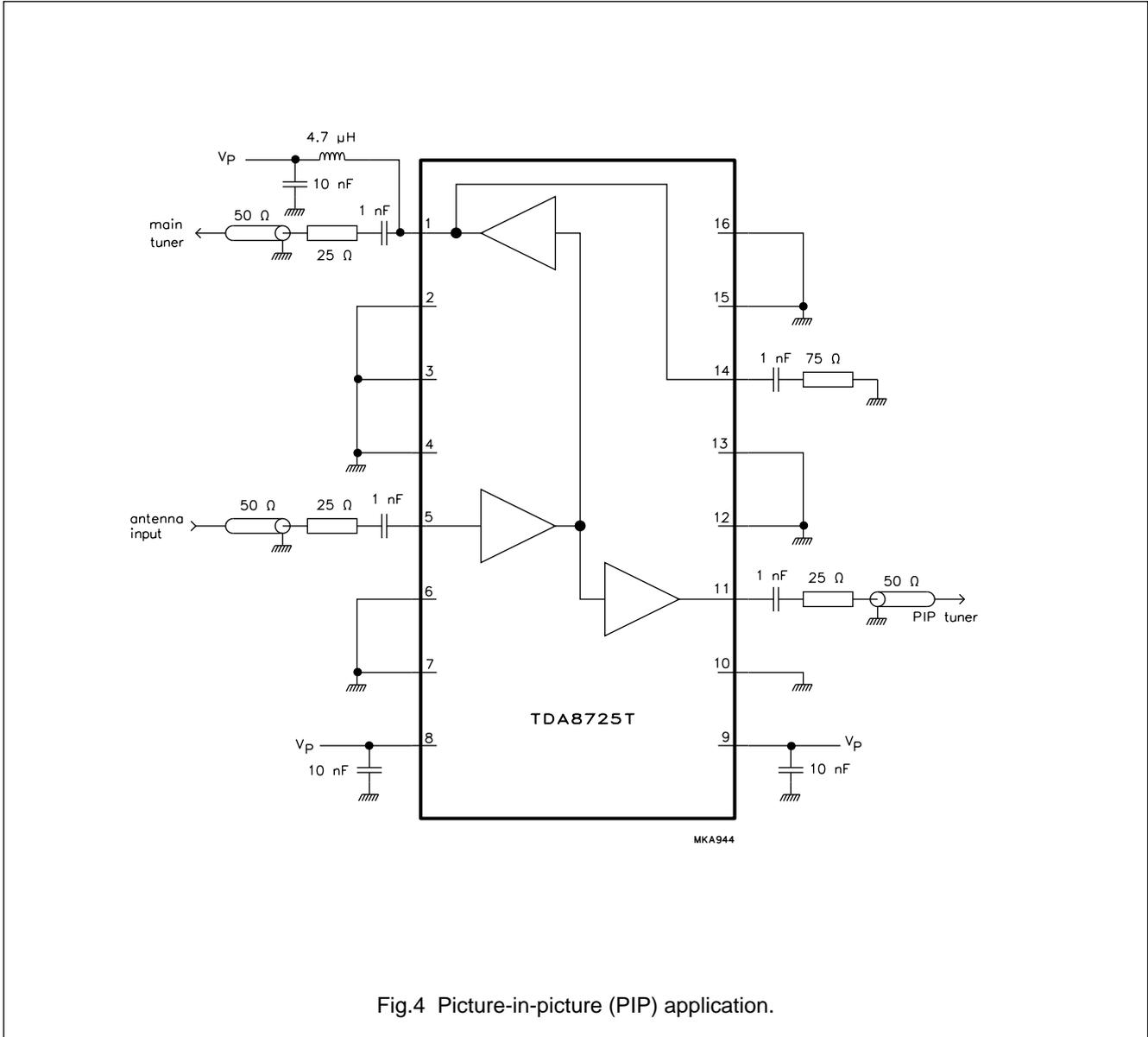
Fig.4 Picture-in-picture (PIP) application.
