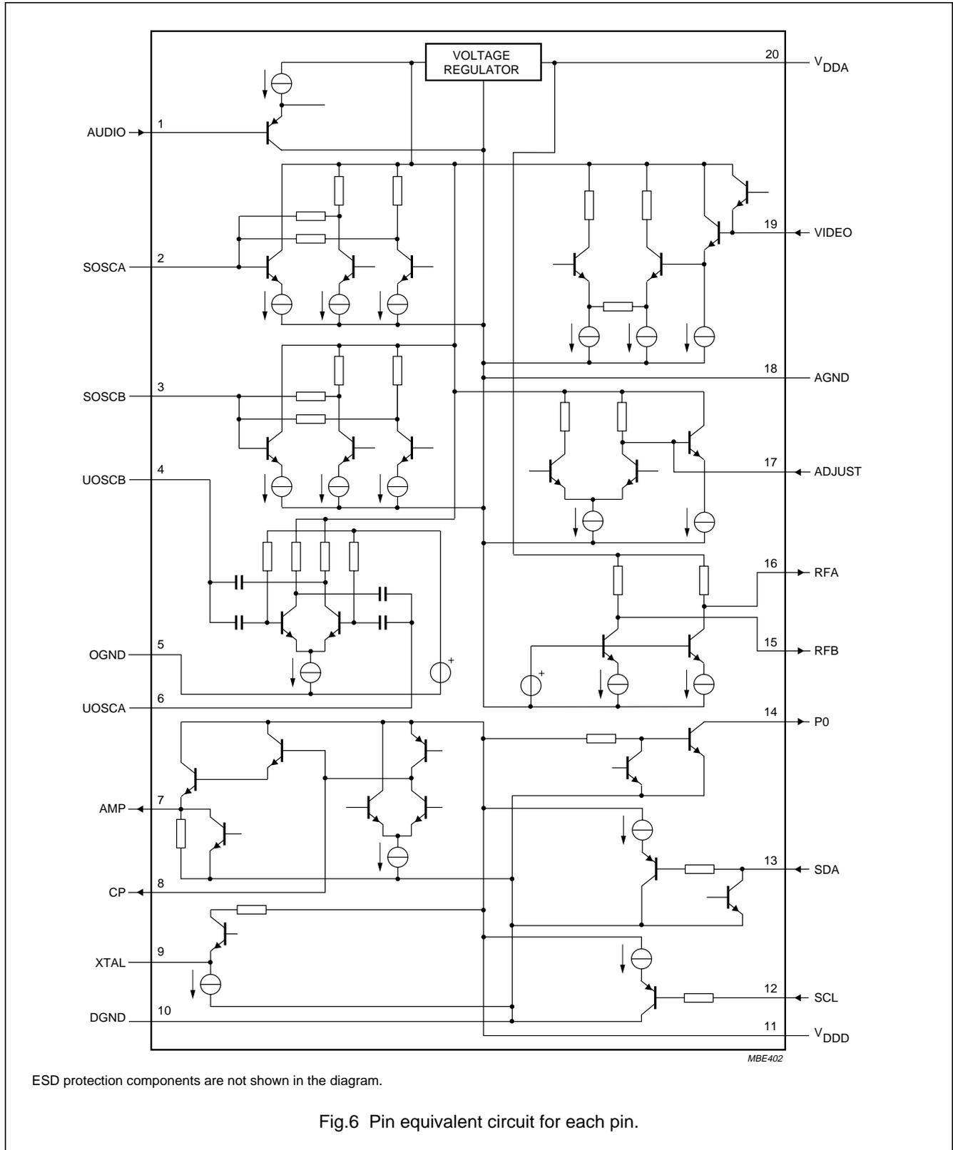
Fig.6 Pin equivalent circuit for each pin.
