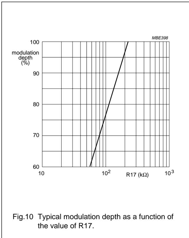
Fig.10 Typical modulation depth as a function of the value of R17.
