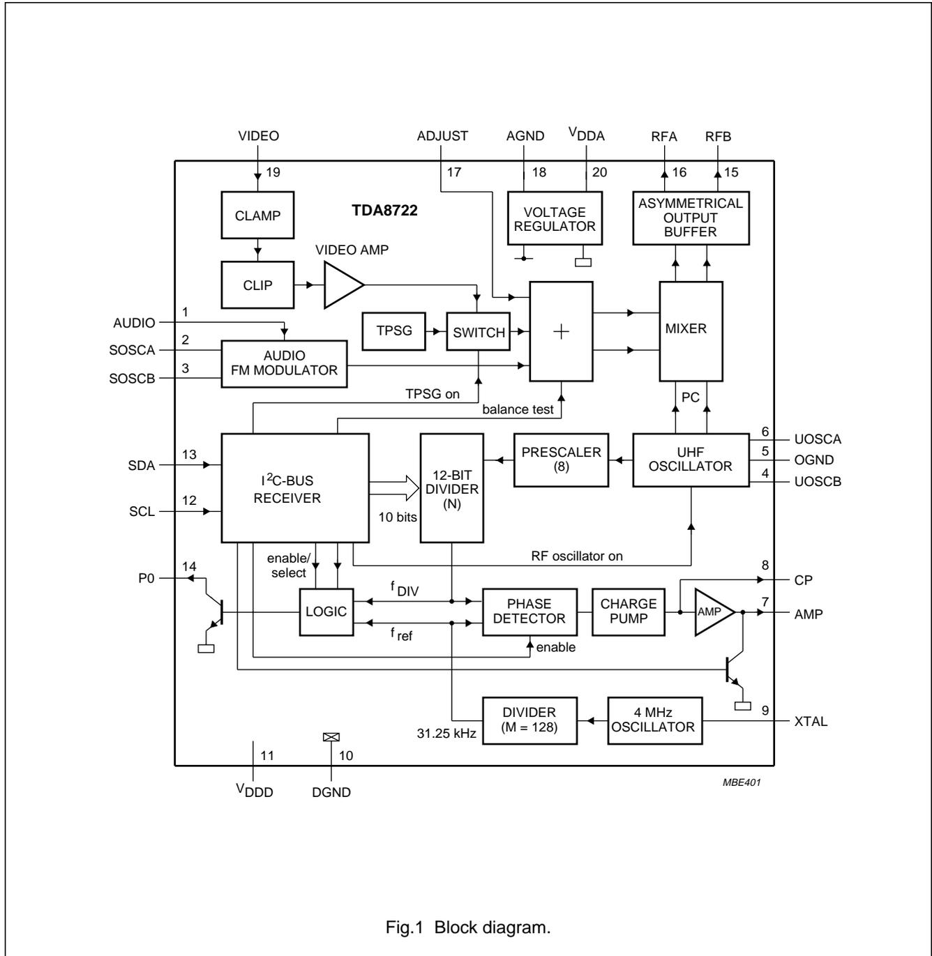
Fig.1 Block diagram.
