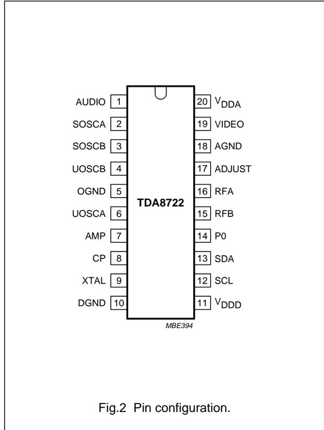
Fig.2 Pin configuration.
