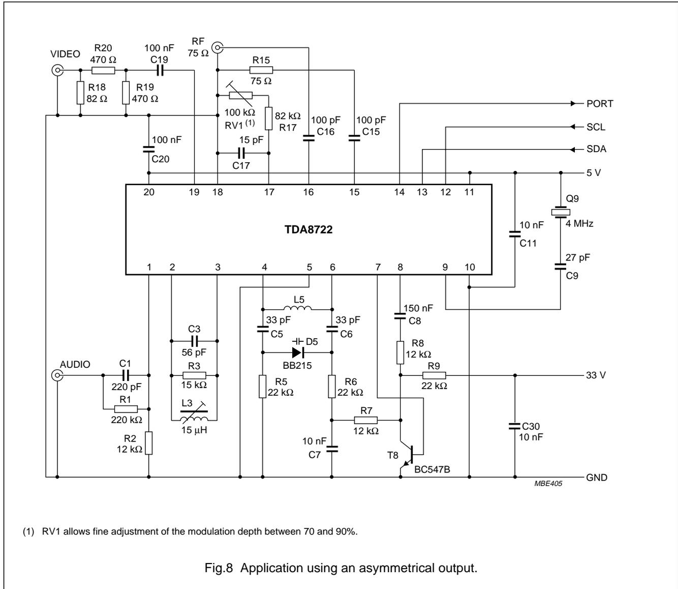
I<sup>2</sup>C-bus programmable modulator for negative video modulation and FM sound
