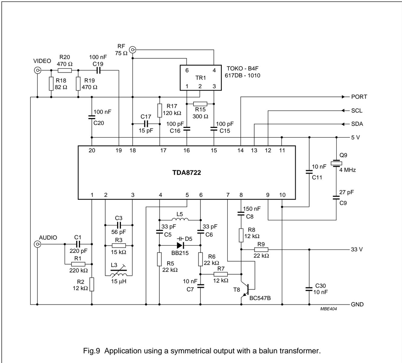
Fig.9 Application using a symmetrical output with a balun transformer.
