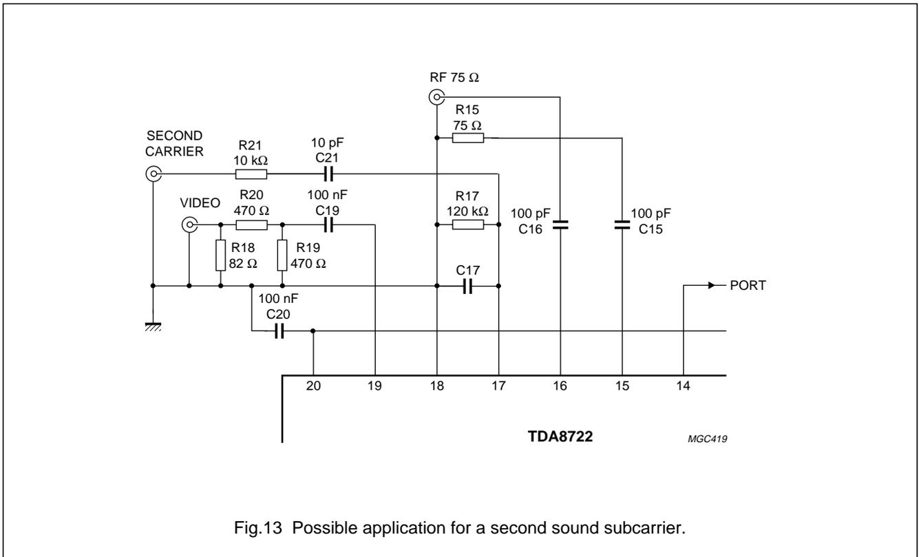
Fig.13 Possible application for a second sound subcarrier.
