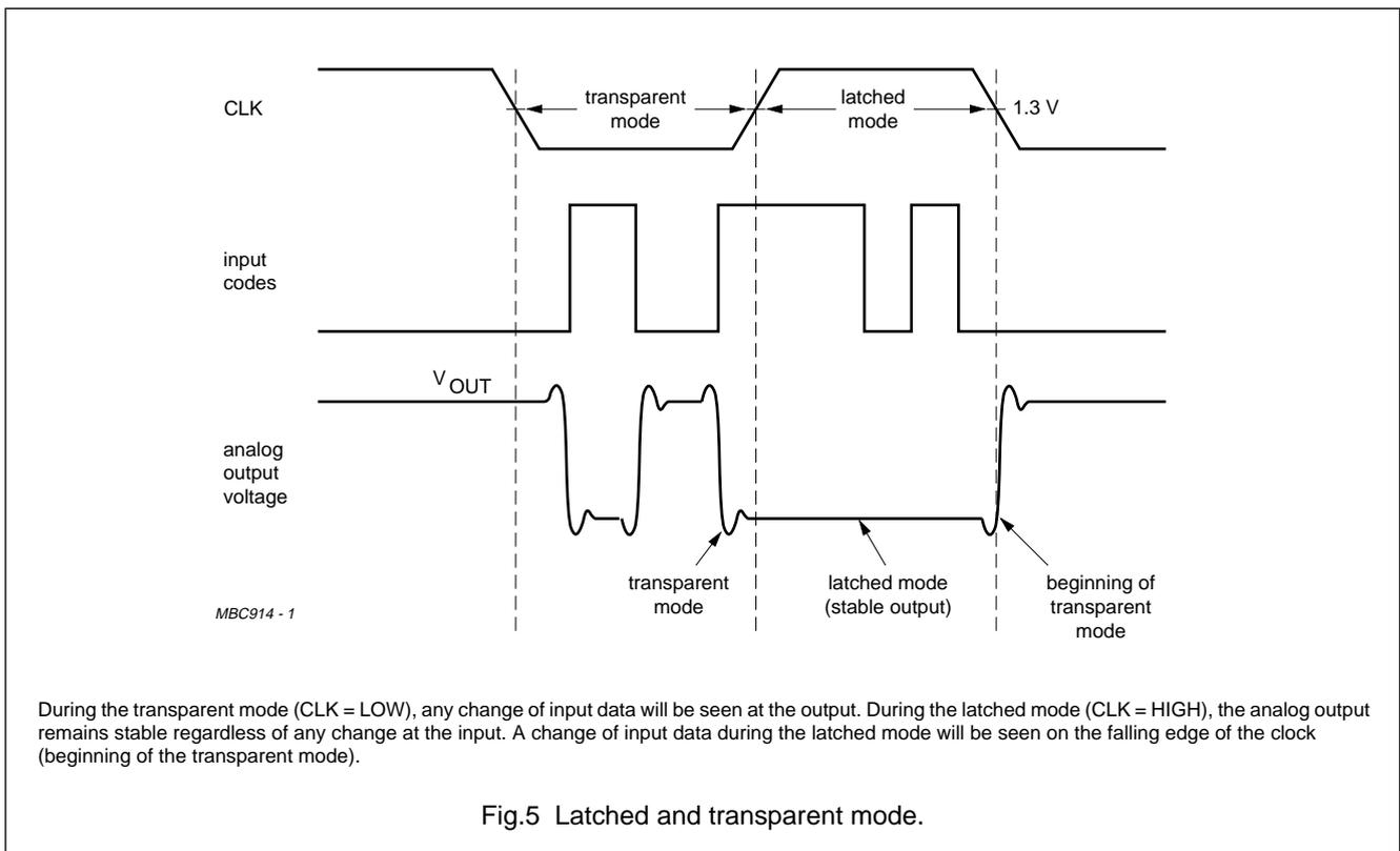
During the transparent mode (CLK = LOW), any change of input data will be seen at the output. During the latched mode (CLK = HIGH), the analog output remains stable regardless of any change at the input. A change of input data during the latched mode will be seen on the falling edge of the clock (beginning of the transparent mode).
