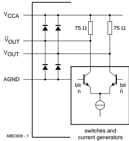
Fig.11 Analog outputs.
