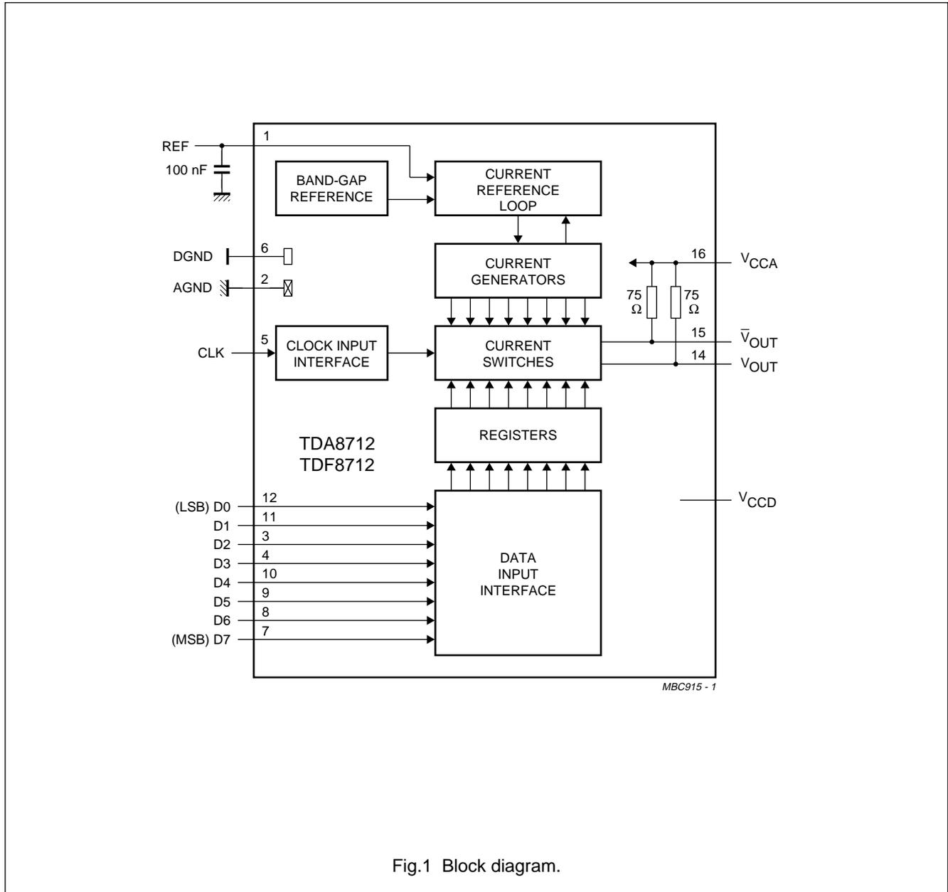
Fig.1 Block diagram.
