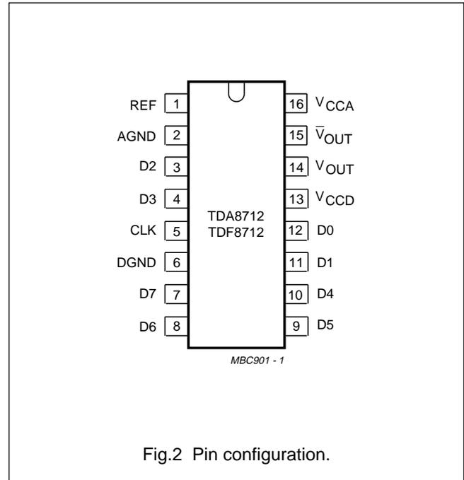
Fig.2 Pin configuration.
