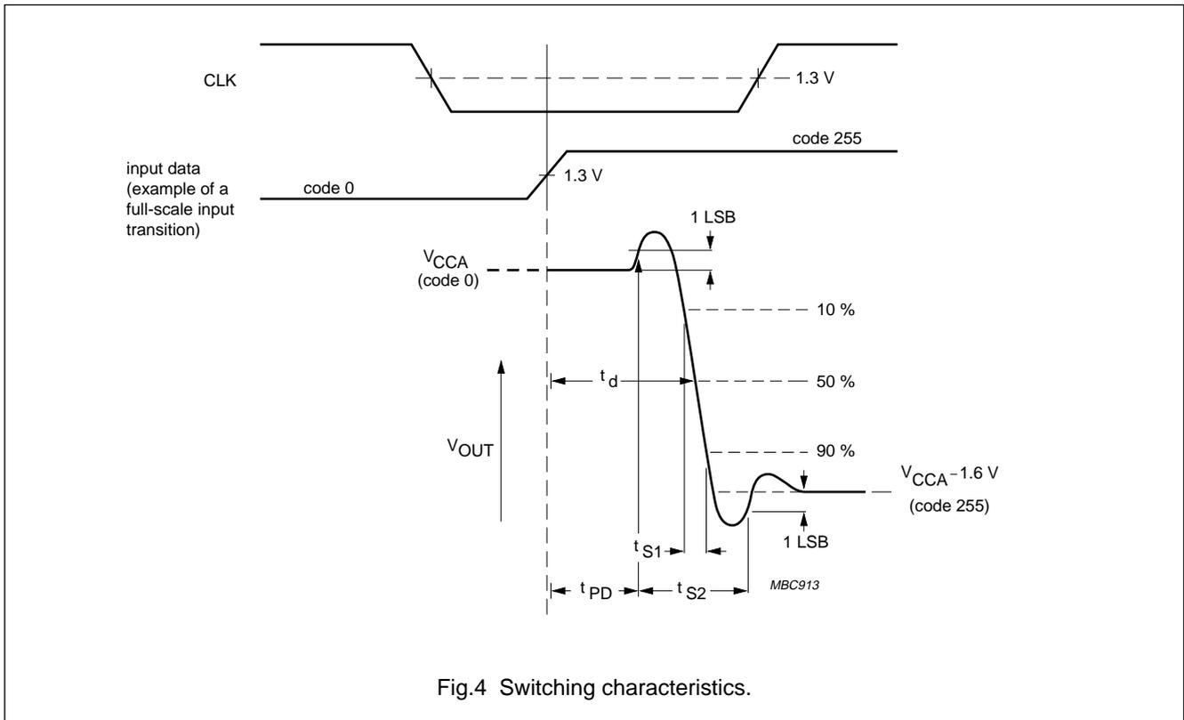
Fig.4 Switching characteristics.
