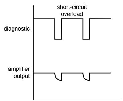
Fig.6 Diagnostic waveform; short-circuit overload.
