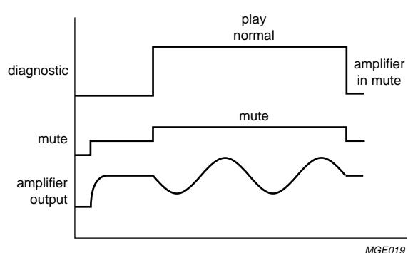
Fig.5 Diagnostic waveform; normal play.
