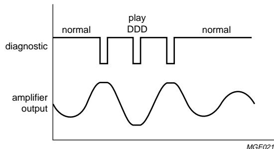
Fig.7 Diagnostic waveform; DDD play.
