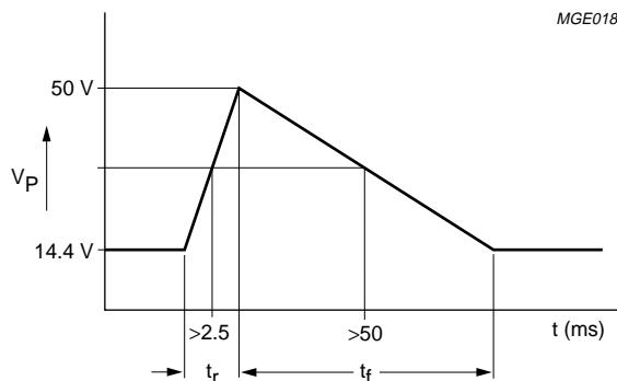
Fig.3 Load dump voltage waveform.
