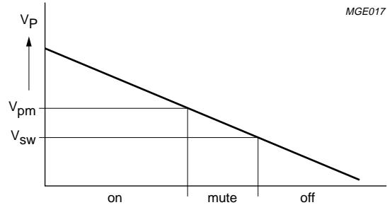
Fig.4 Low voltage supply behaviour.
