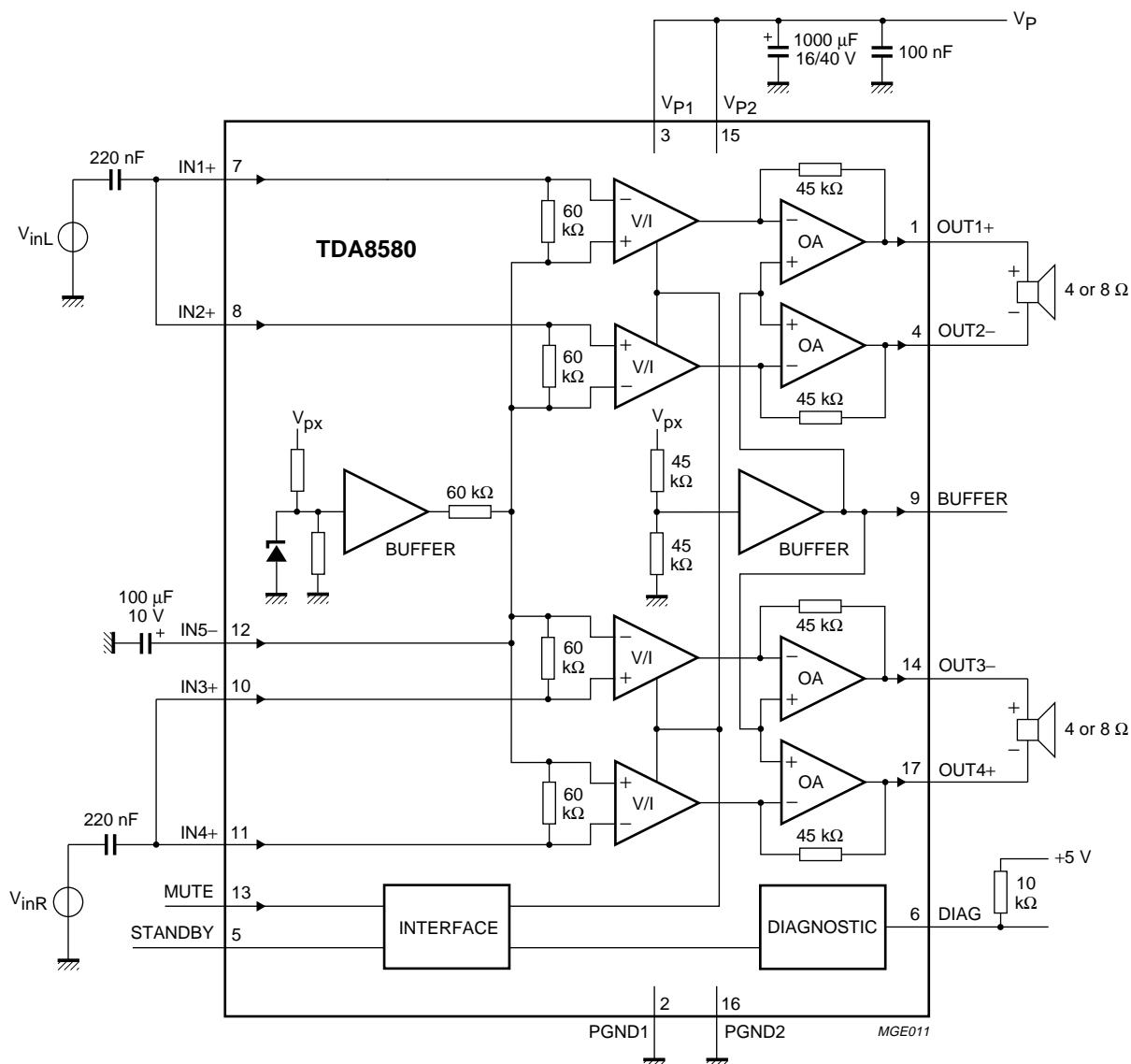
Fig.9 Stereo bridge-tied load application.
