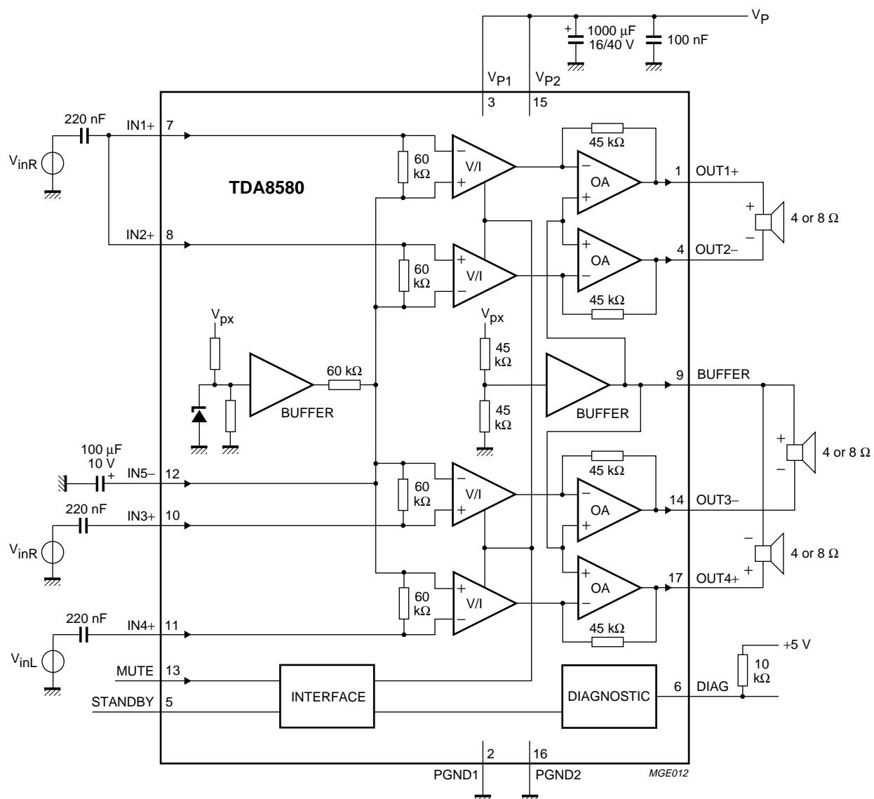
Fig.11 Dual single-ended and one bridge-tied load application.
