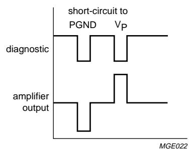
Fig.8 Diagnostic waveform; short-circuit to GND and V<sub>P</sub>.
