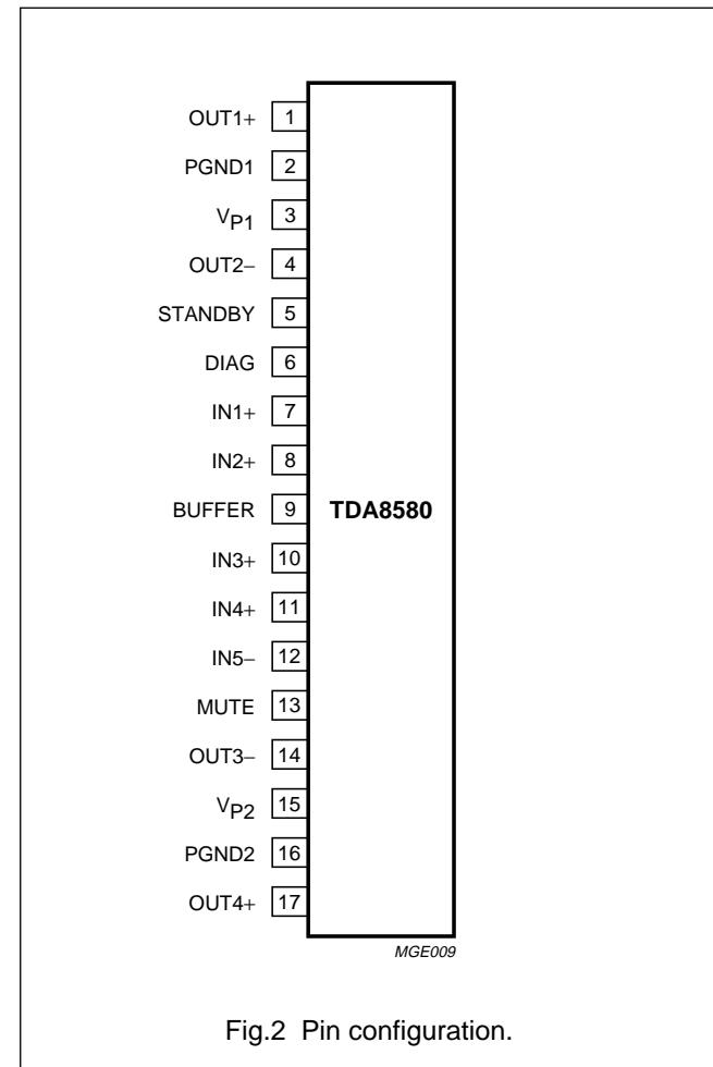
Fig.2 Pin configuration.
