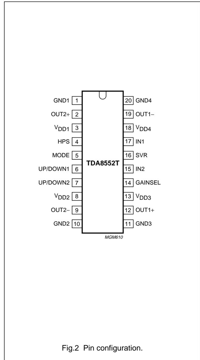
Fig.2 Pin configuration.
