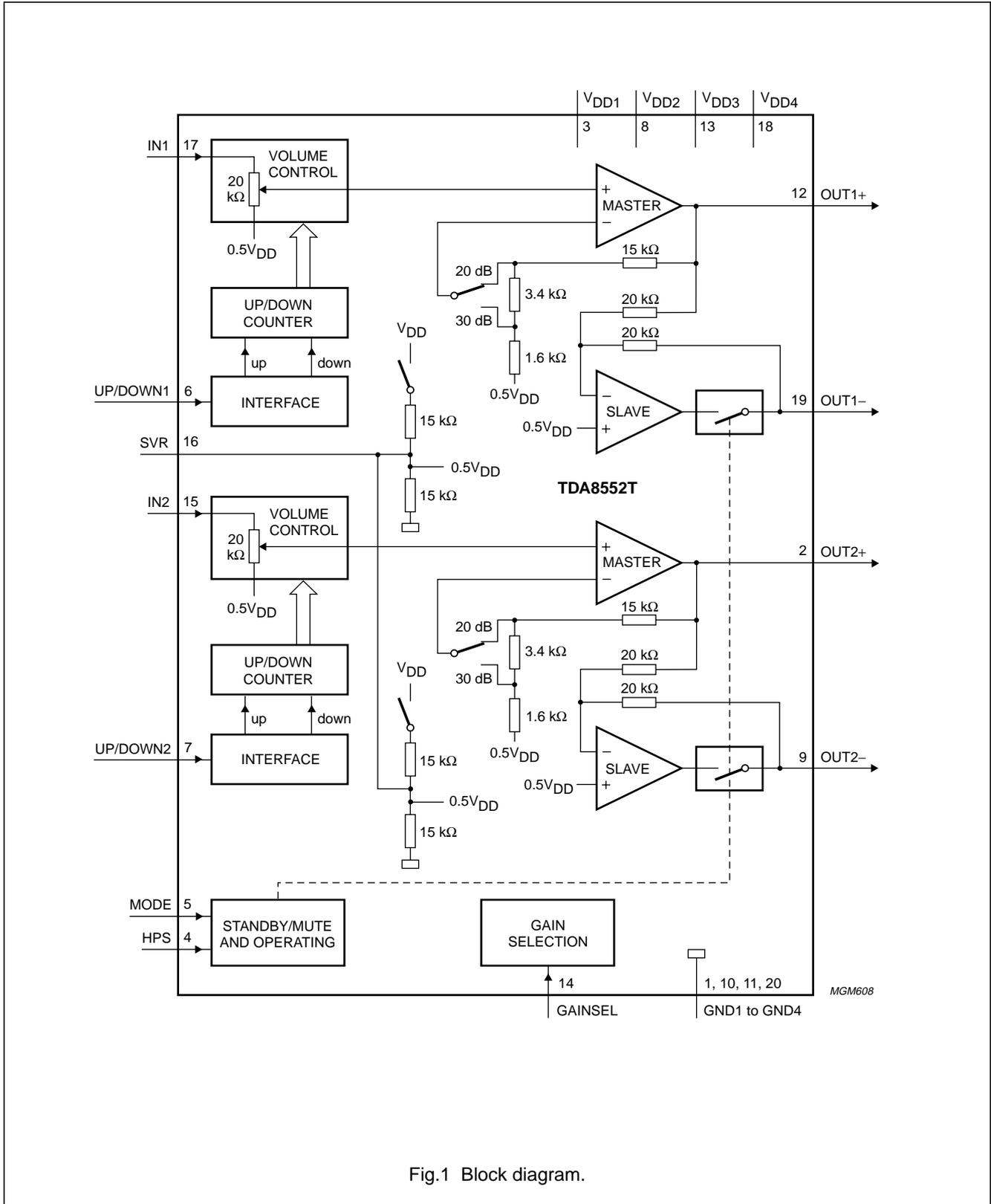
Fig.1 Block diagram.
