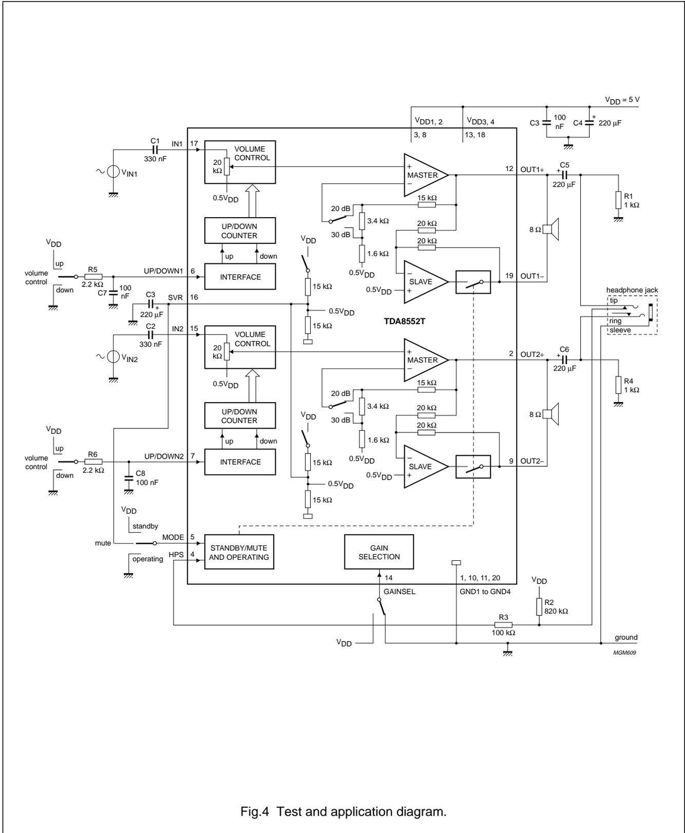
Fig.4 Test and application diagram.
