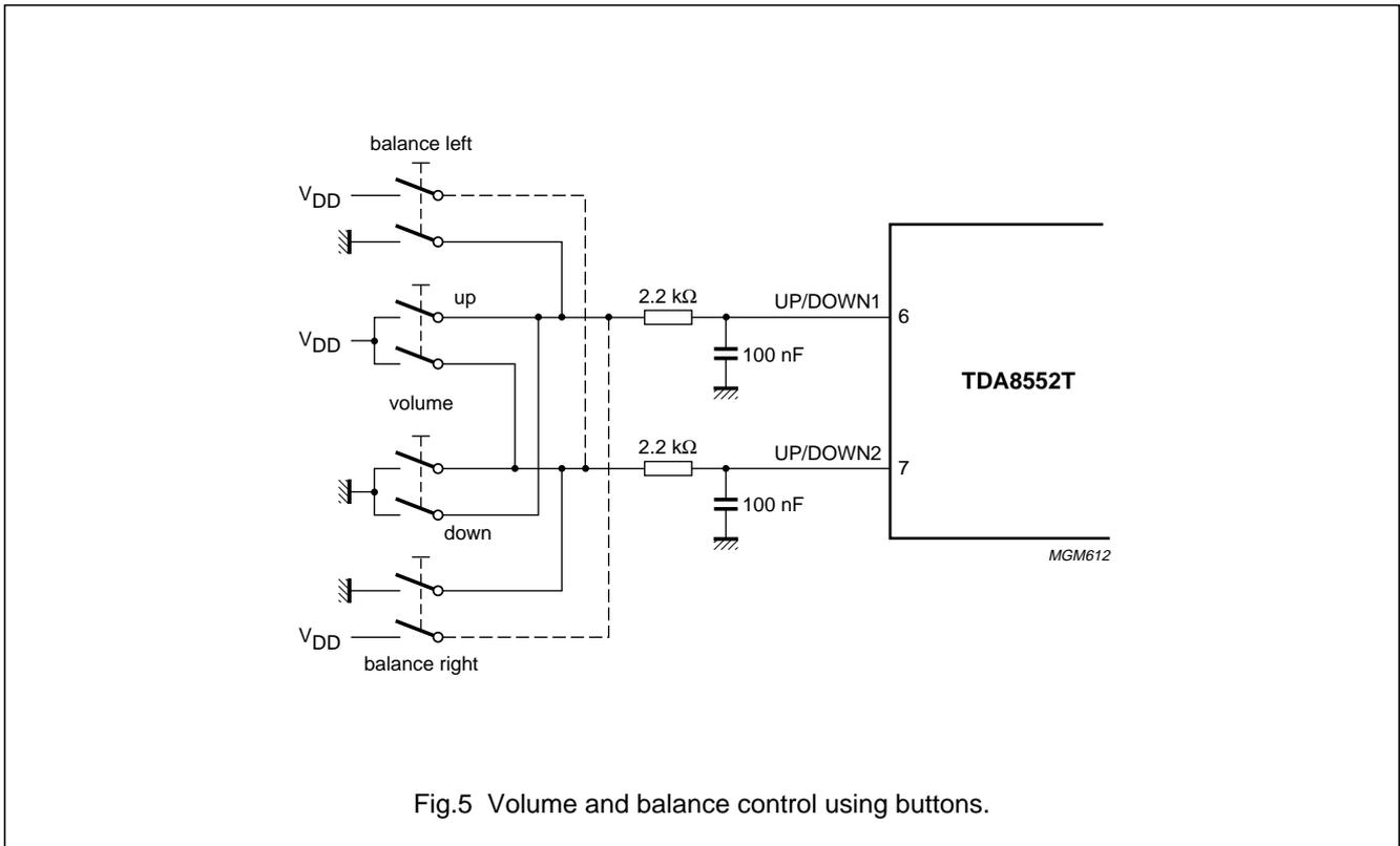
Fig.5 Volume and balance control using buttons.
