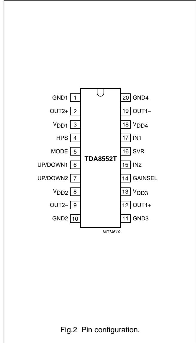
Fig.2 Pin configuration.
