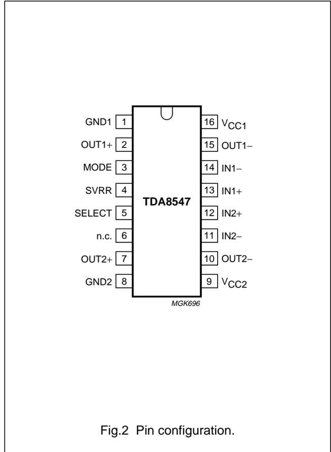
Fig.2 Pin configuration.
