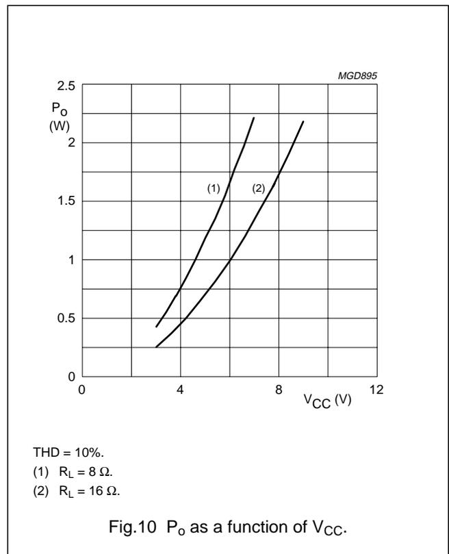
2 × 1 W BTL audio amplifier with output channel switching
