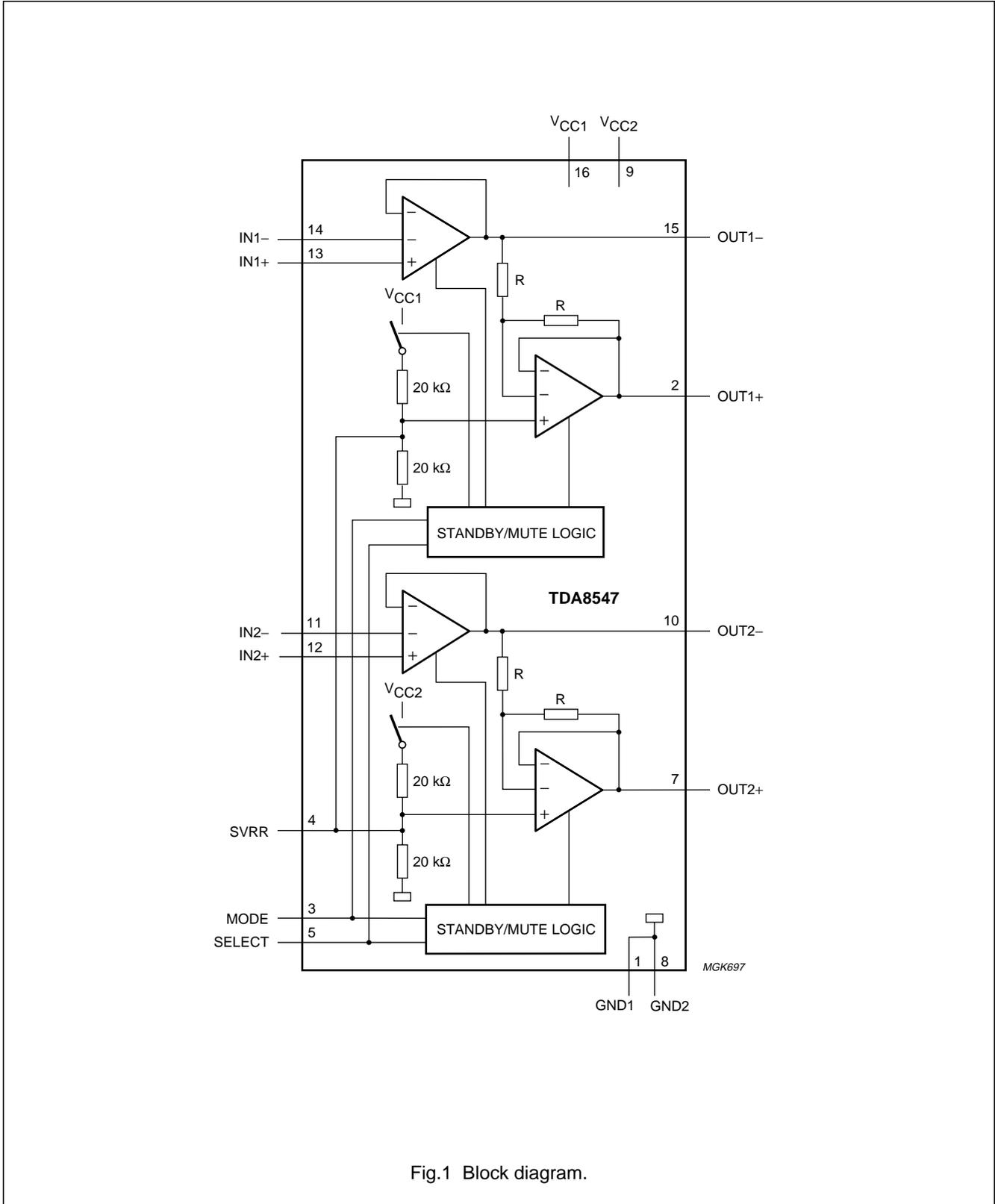
Fig.1 Block diagram.
