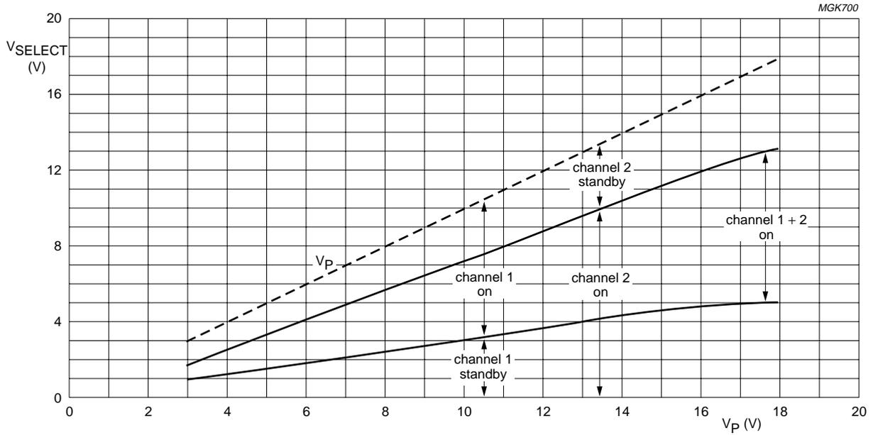
Fig.15  $V_{SELECT}$  as a function of  $V_P$ .
