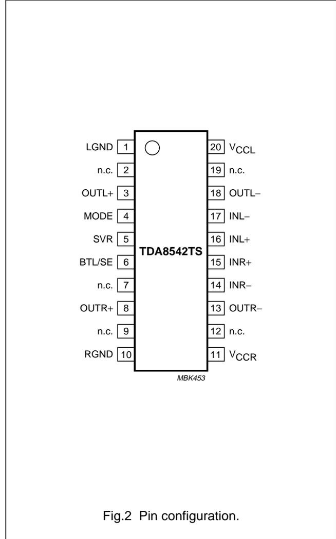
Fig.2 Pin configuration.
