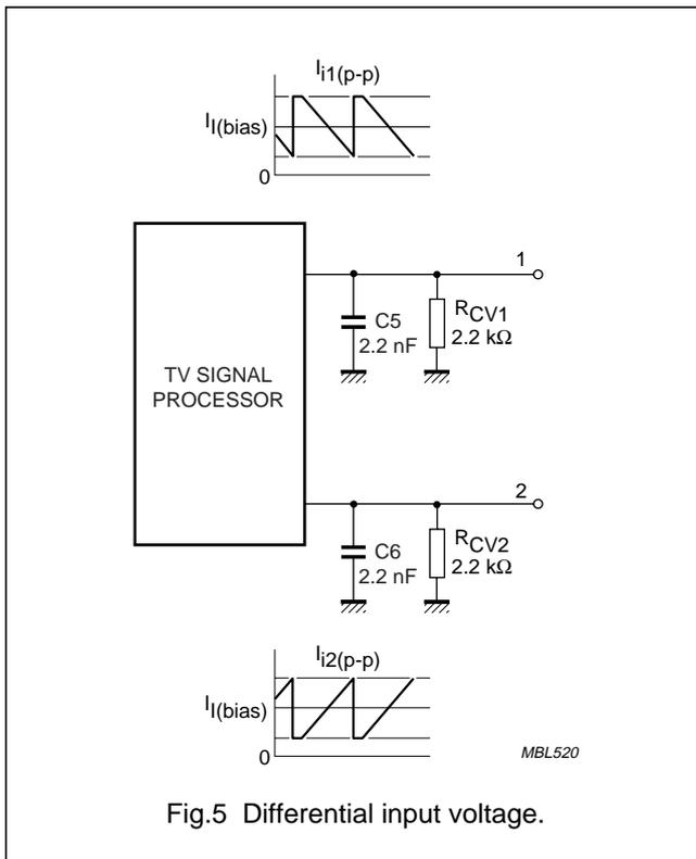
Fig.5 Differential input voltage.
