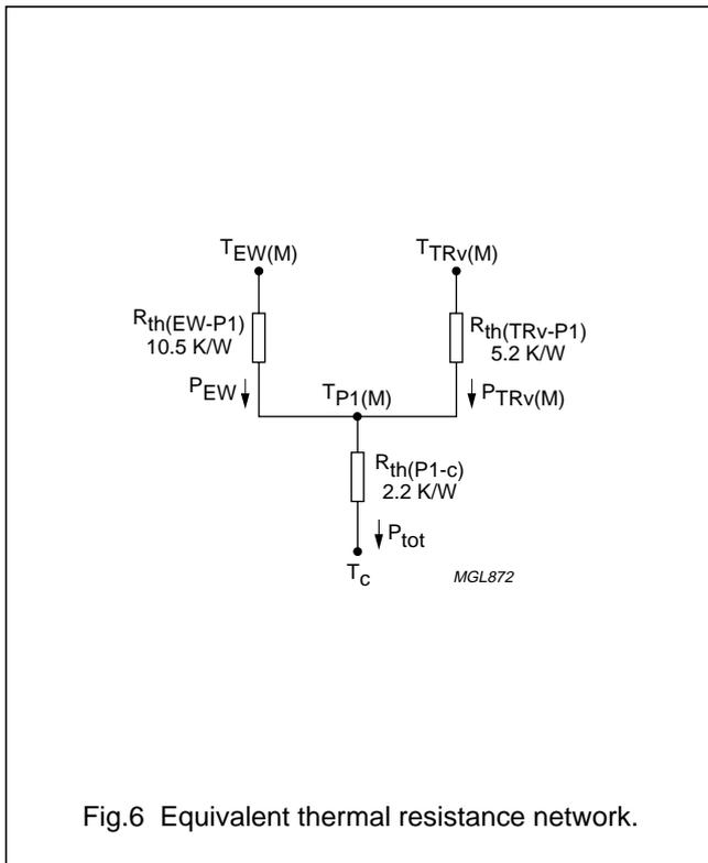
Fig.6 Equivalent thermal resistance network.
