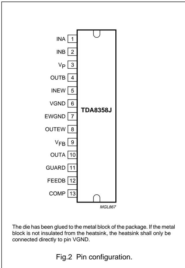
Fig.2 Pin configuration.
