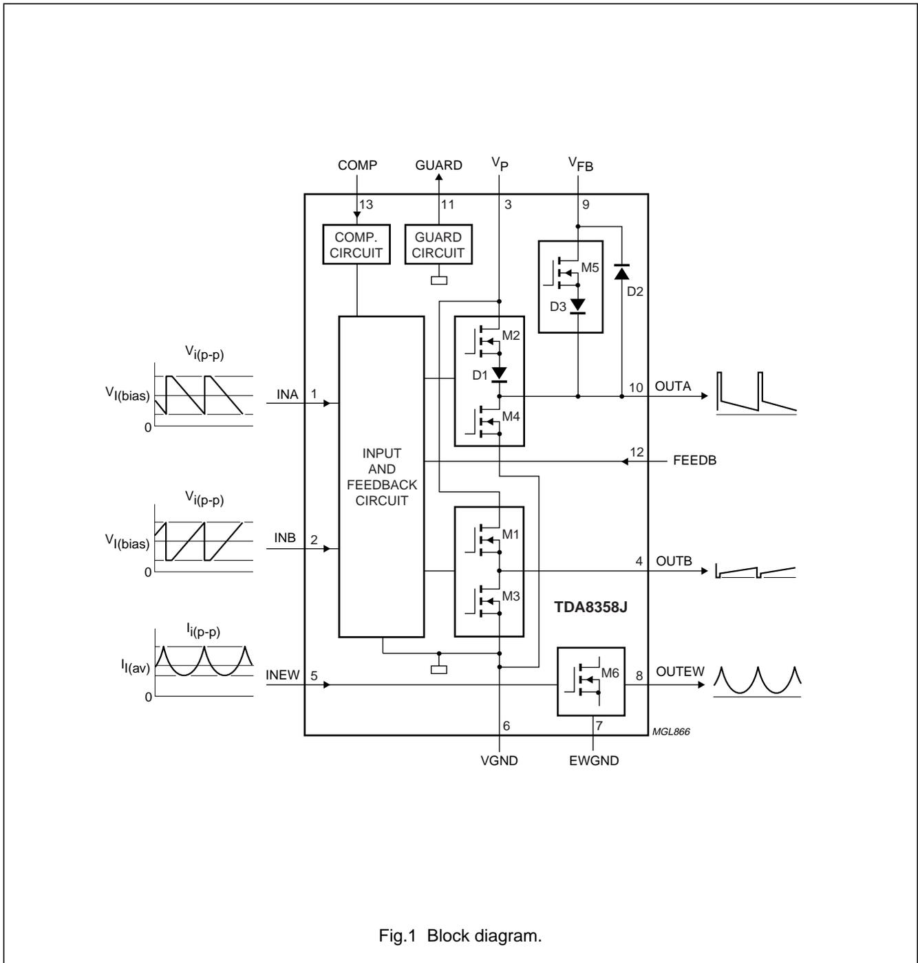
Fig.1 Block diagram.
