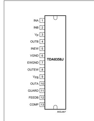
The die has been glued to the metal block of the package. If the metal block is not insulated from the heatsink, the heatsink shall only be connected directly to pin VGND.
