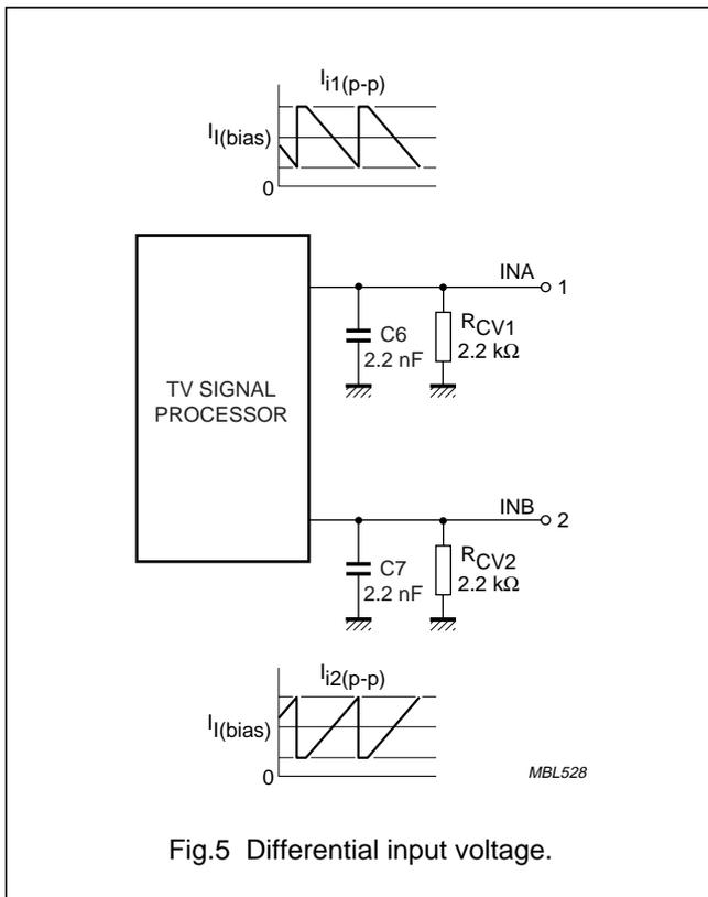
Fig.5 Differential input voltage.
