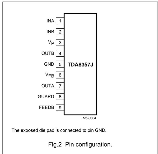
Fig.2 Pin configuration.
