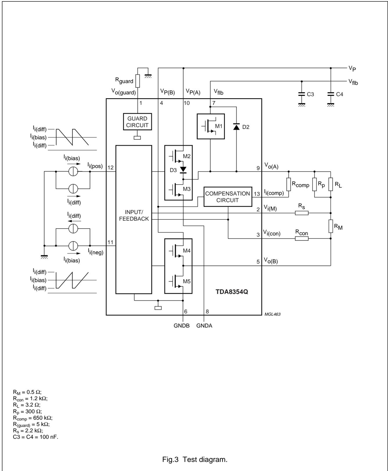
Fig.3 Test diagram.
