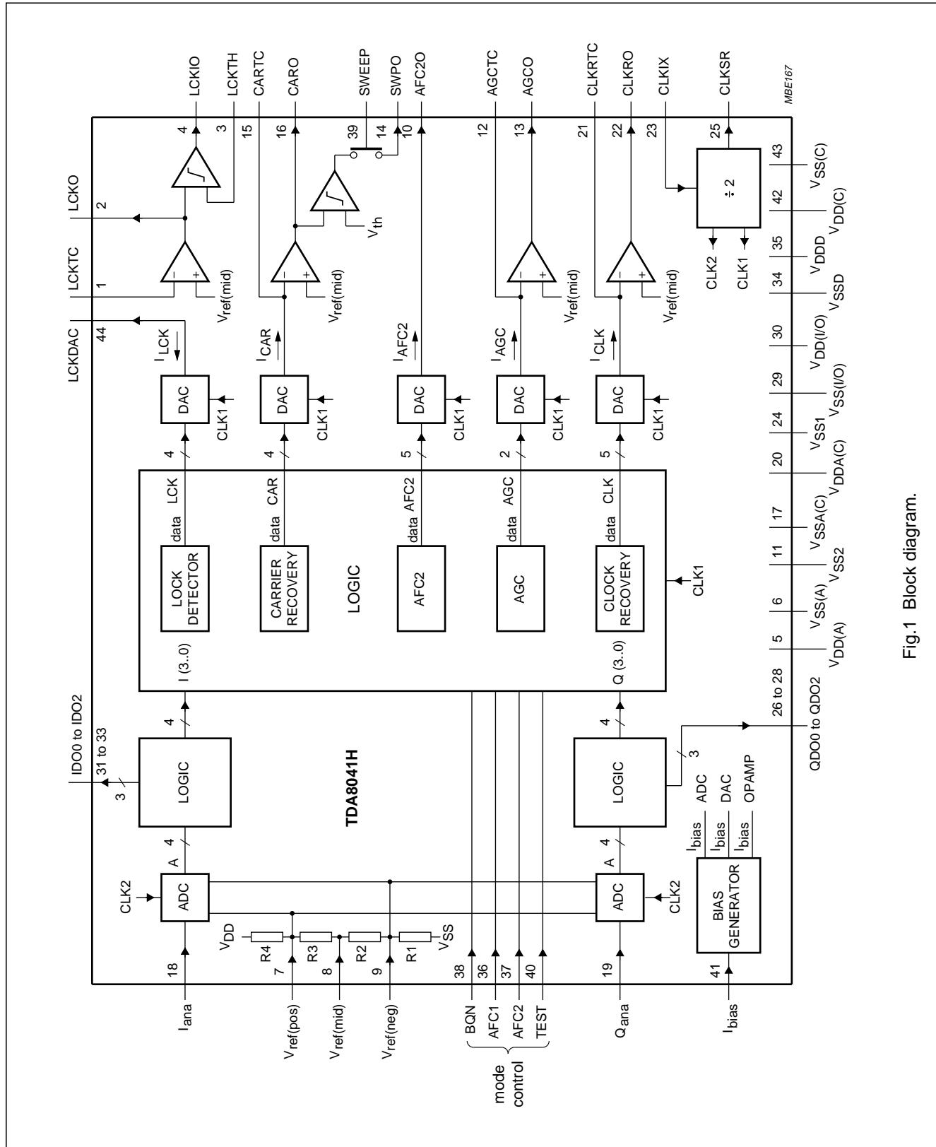
Fig.1 Block diagram.
