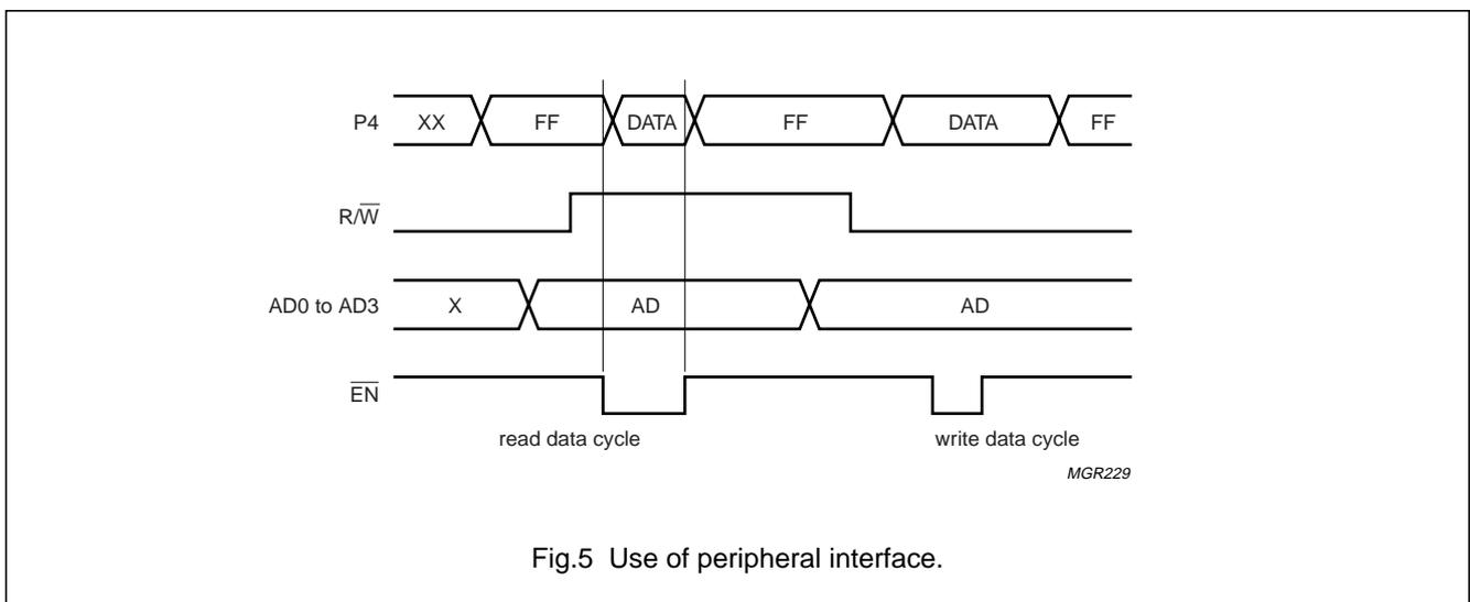
Fig.5 Use of peripheral interface.
