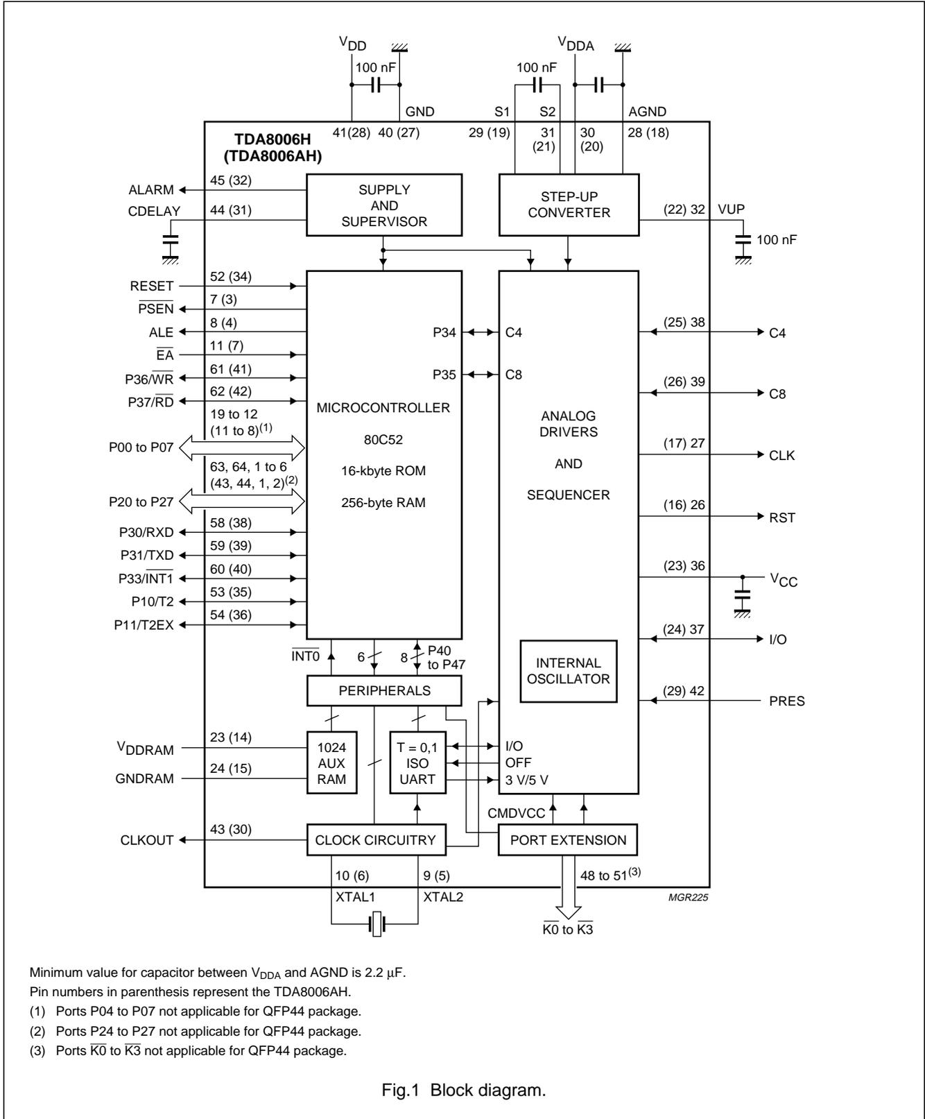
Minimum value for capacitor between V<sub>DDA</sub> and AGND is 2.2 μF.
