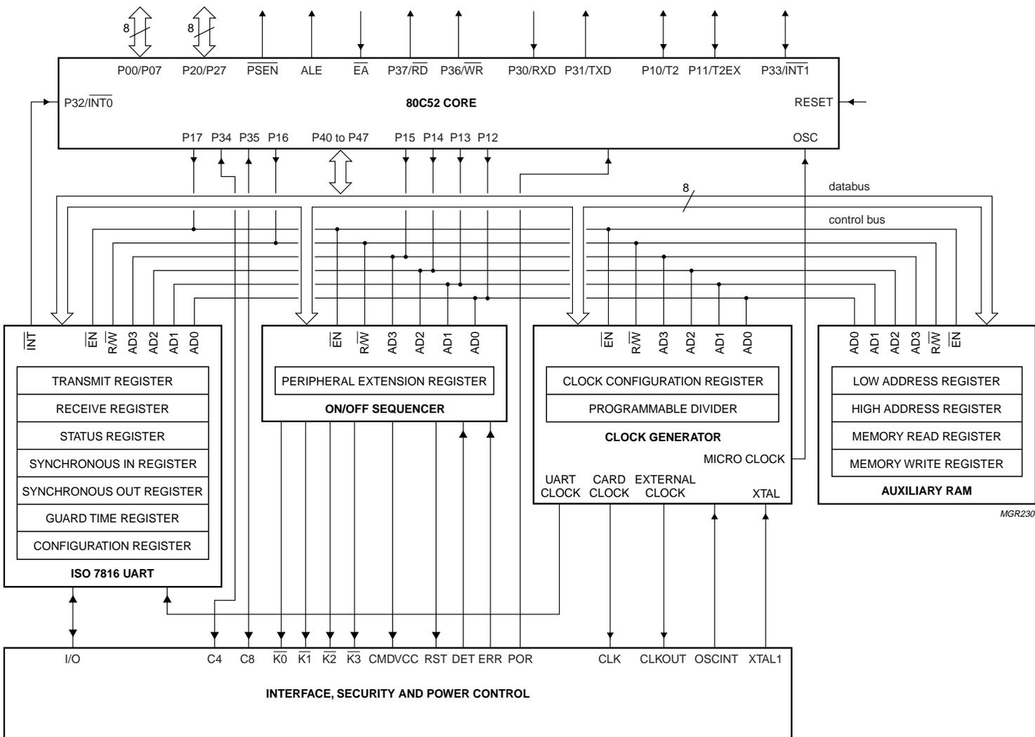
Fig.6 Peripheral interface.
