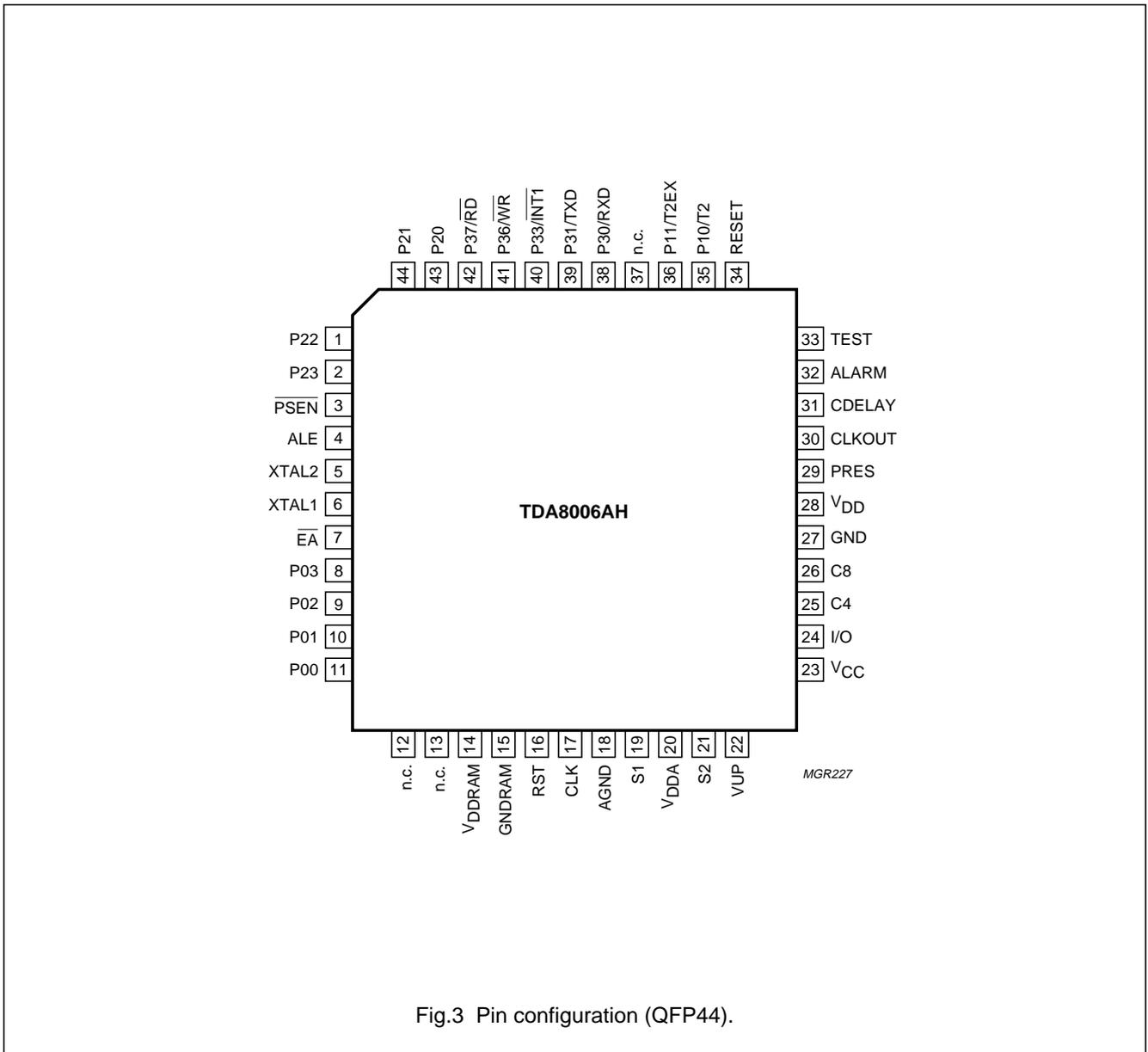
Fig.3 Pin configuration (QFP44).
