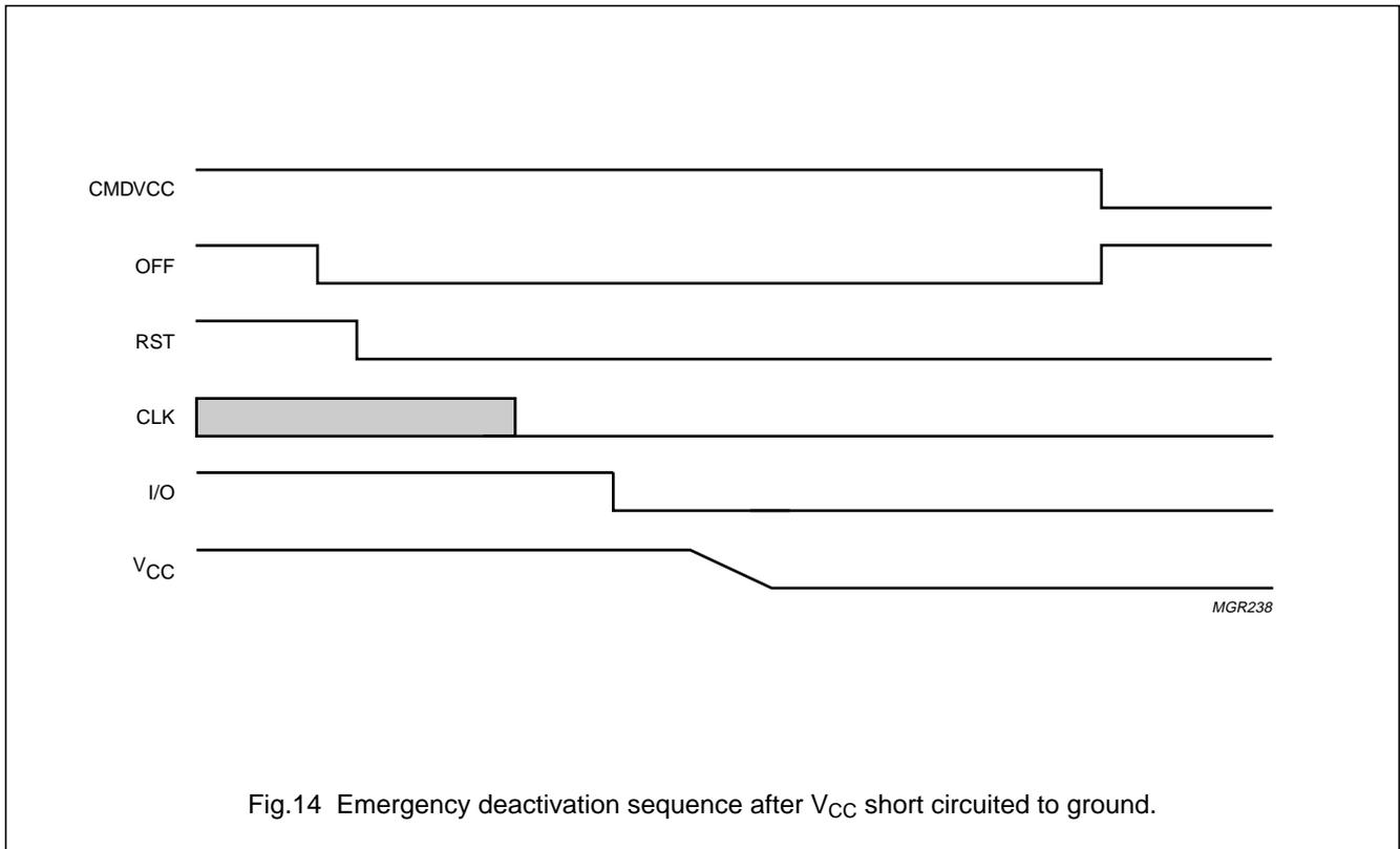
Fig.14 Emergency deactivation sequence after V<sub>CC</sub> short circuited to ground.
