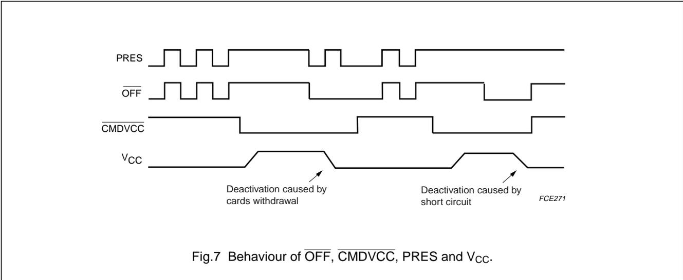
Fig.7 Behaviour of  $\overline{\text{OFF}}$ ,  $\overline{\text{CMDVCC}}$ , PRES and  $V_{\text{CC}}$ .
