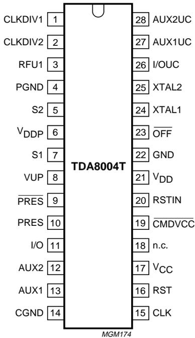
Fig.2 Pin configuration.
