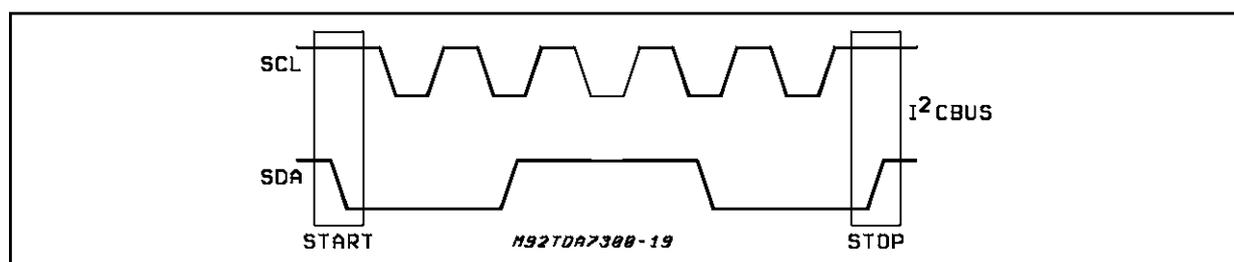
Figure 5: Acknowledge on the I<sup>2</sup>CBUS
