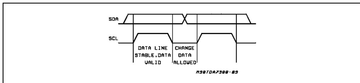
Figure 4: Timing Diagram of I<sup>2</sup>CBUS
