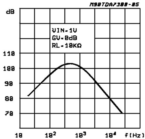
Figure 9: Input Separation (L1 - L2) vs. Frequency
