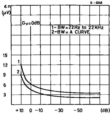
Figure 4: Signal to Noise Ratio vs. Volume Setting
