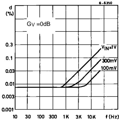
Figure 6: Distortion vs. Output Voltage
