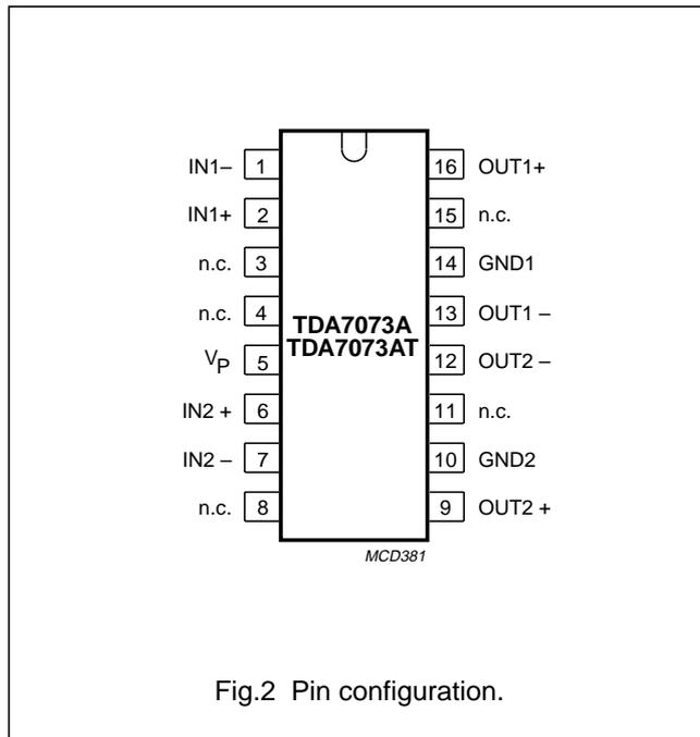
Fig.2 Pin configuration.
