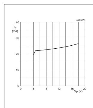
Fig.3 Quiescent current as a function of supply voltage.
