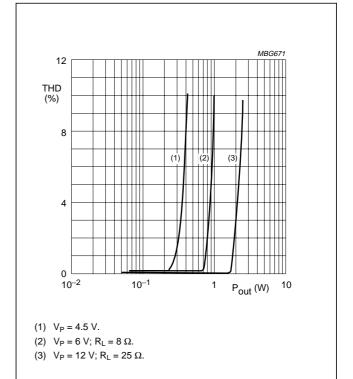
Fig.4 THD as a function of output power.
