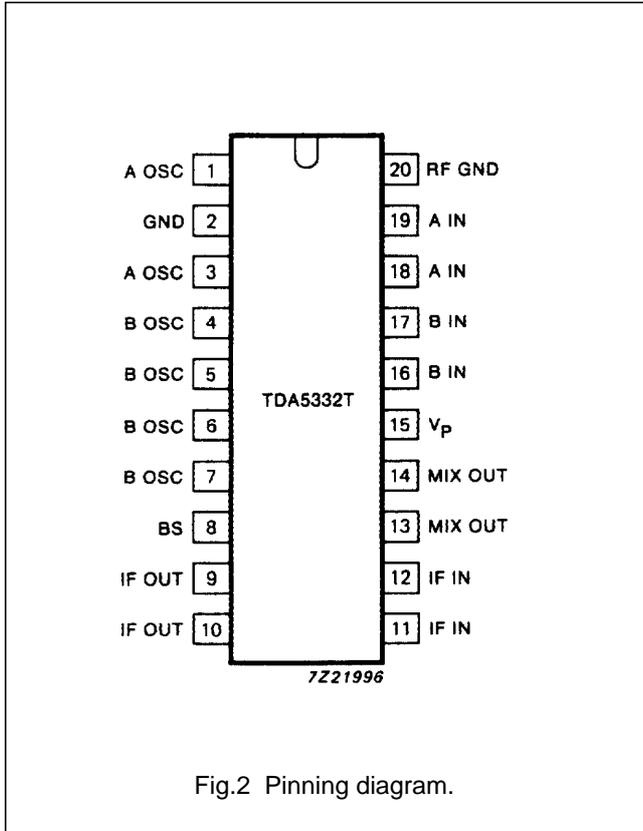
Fig.2 Pinning diagram.
