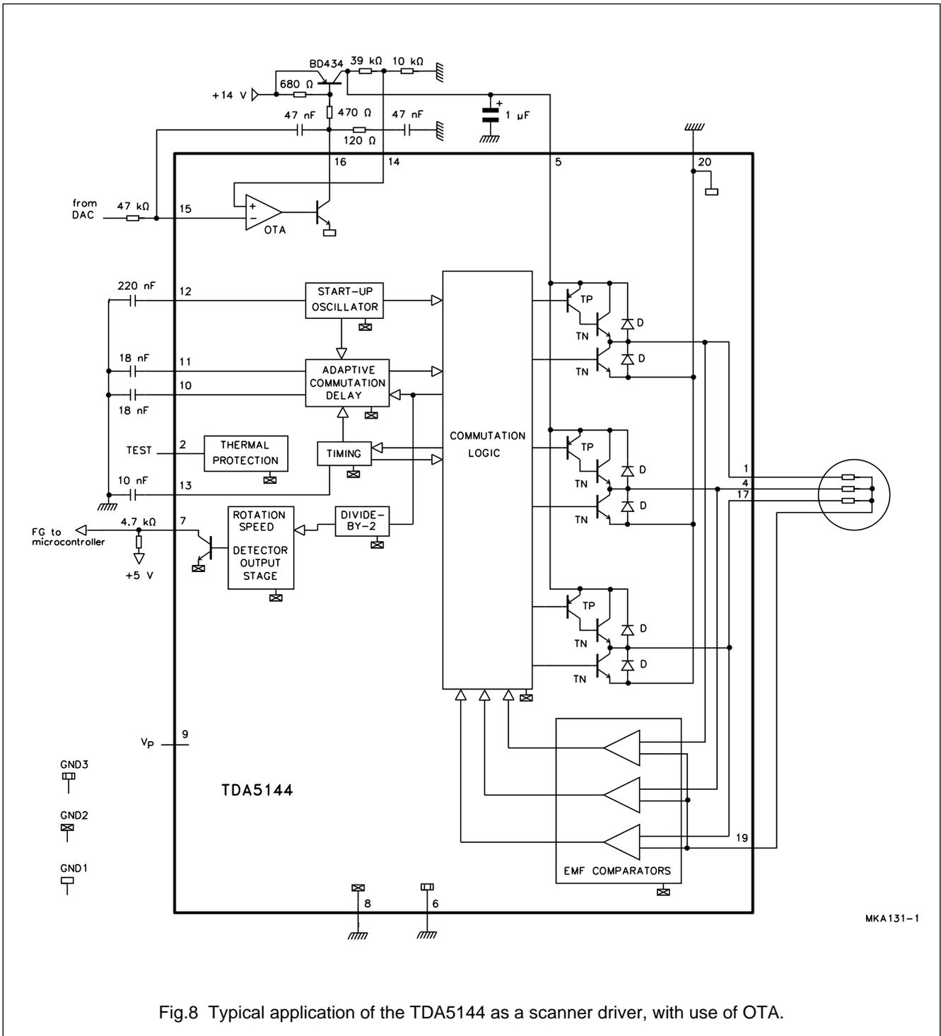
Fig.8 Typical application of the TDA5144 as a scanner driver, with use of OTA.
