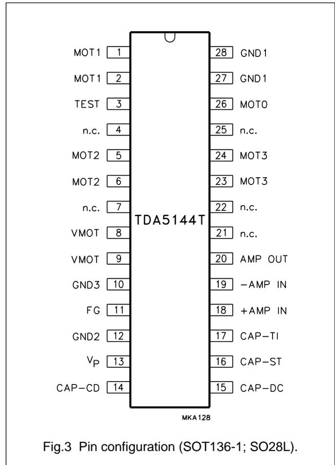
Fig.3 Pin configuration (SOT136-1; SO28L).
