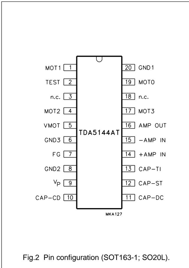
Fig.2 Pin configuration (SOT163-1; SO20L).
