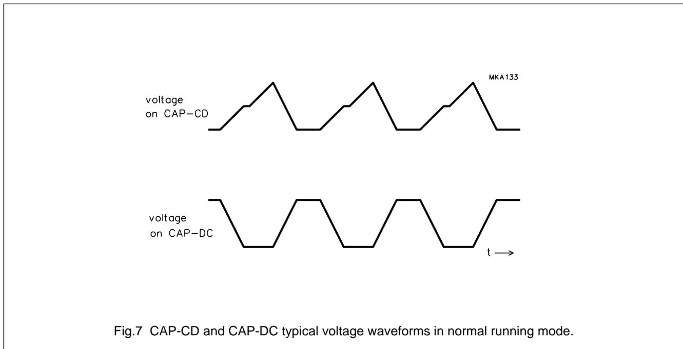
Fig.7 CAP-CD and CAP-DC typical voltage waveforms in normal running mode.
