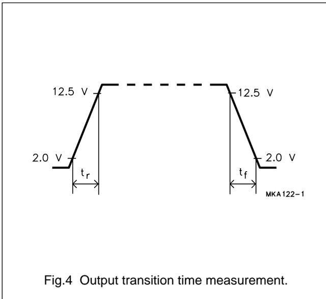
Fig.4 Output transition time measurement.
