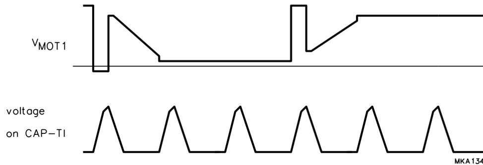
If the chosen value of CAP-TI is too small oscillations can occur in certain positions of a blocked rotor. If the chosen value is too large, then it is possible that the motor may run in the reverse direction (synchronously with little torque).
