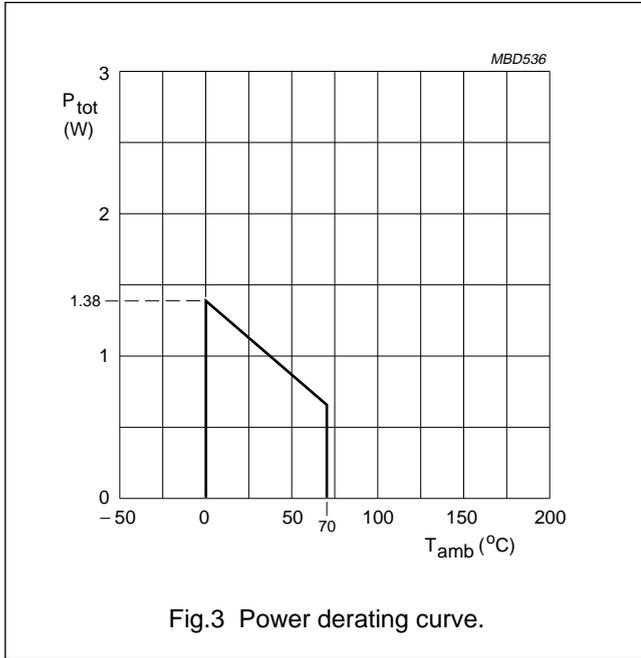
Fig.3 Power derating curve.
