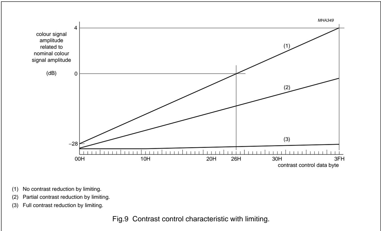
150 MHz video controller with I<sup>2</sup>C-bus
