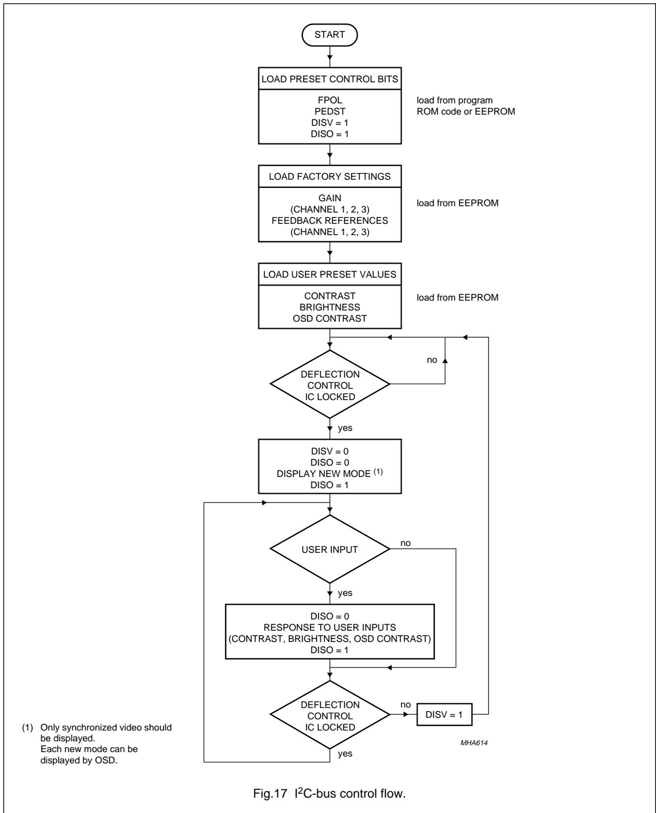
Fig.17 I<sup>2</sup>C-bus control flow.
