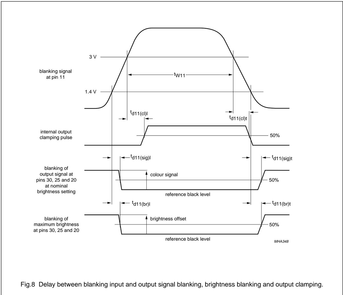
Fig.8 Delay between blanking input and output signal blanking, brightness blanking and output clamping.
