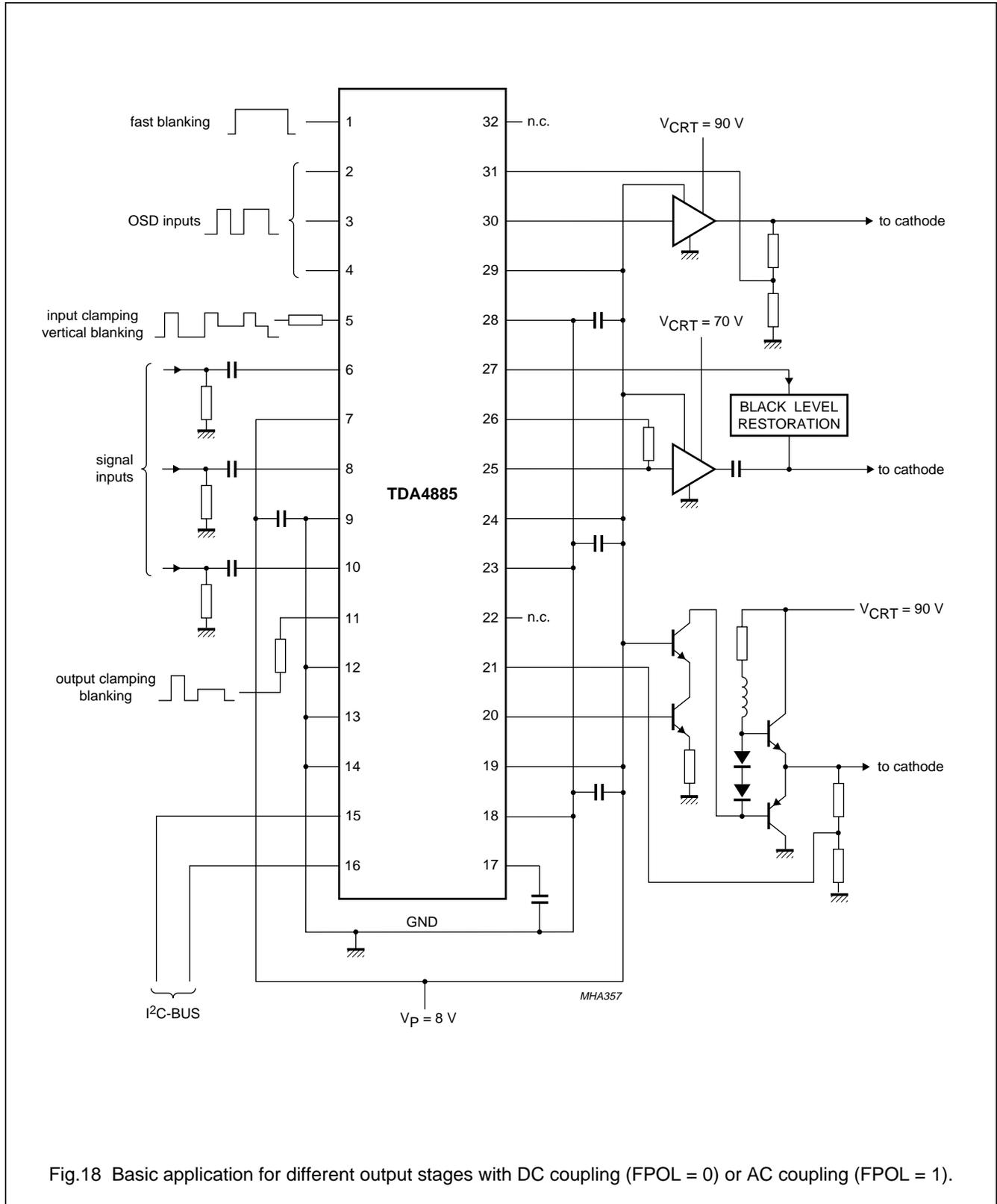
Fig.18 Basic application for different output stages with DC coupling (FPOL = 0) or AC coupling (FPOL = 1).
