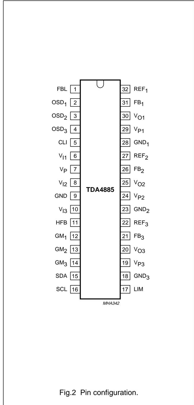
150 MHz video controller with I<sup>2</sup>C-bus
