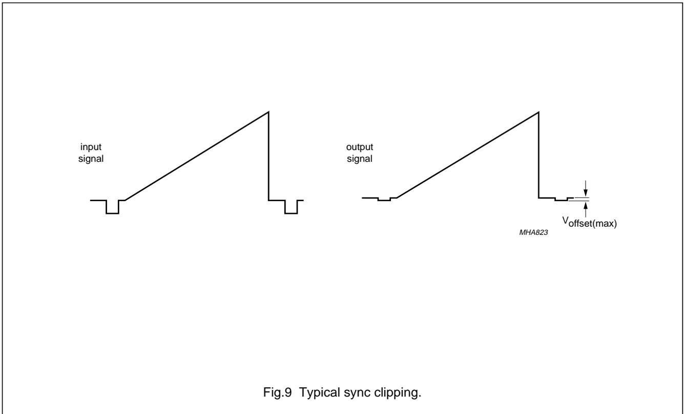
Fig.9 Typical sync clipping.
