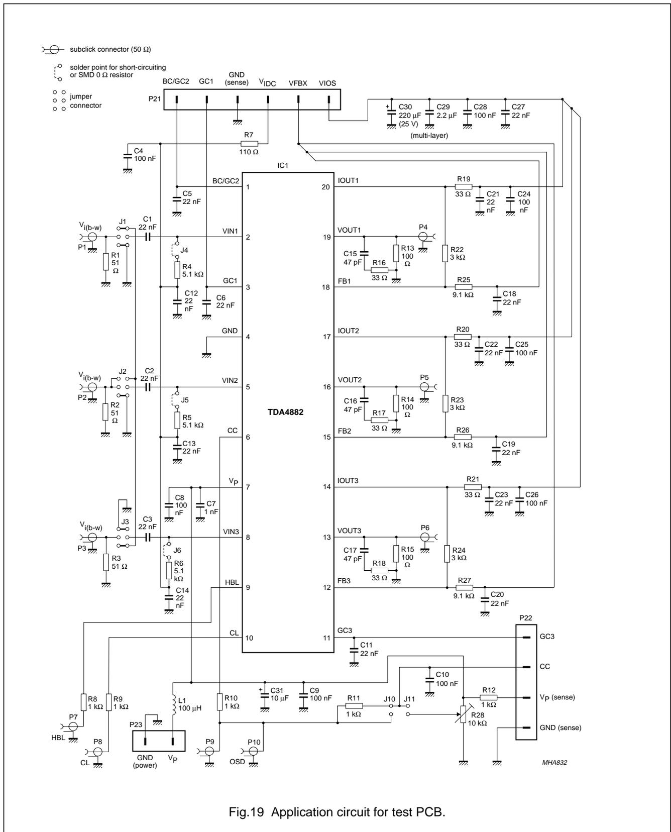
Fig.19 Application circuit for test PCB.
