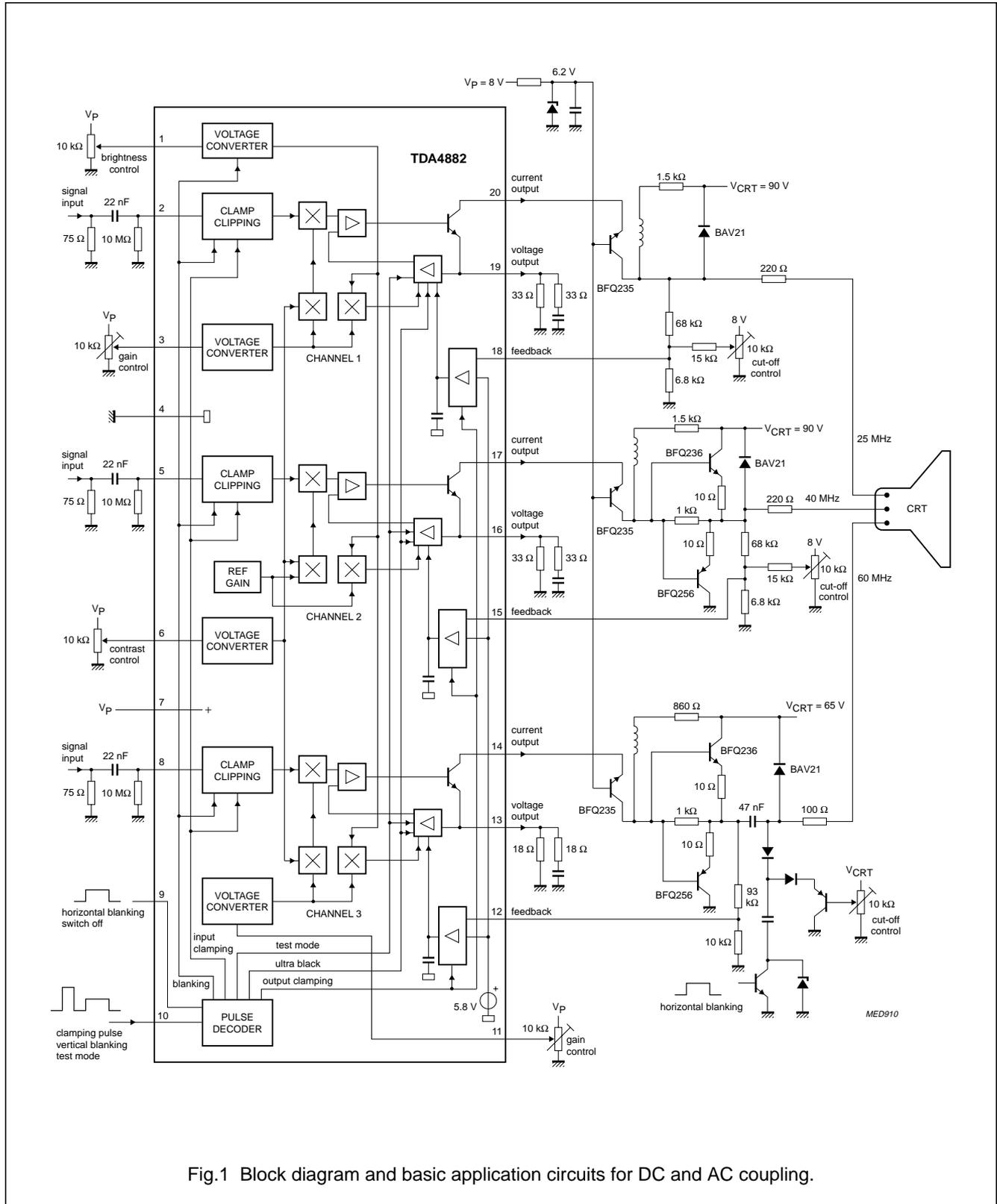
Fig.1 Block diagram and basic application circuits for DC and AC coupling.
