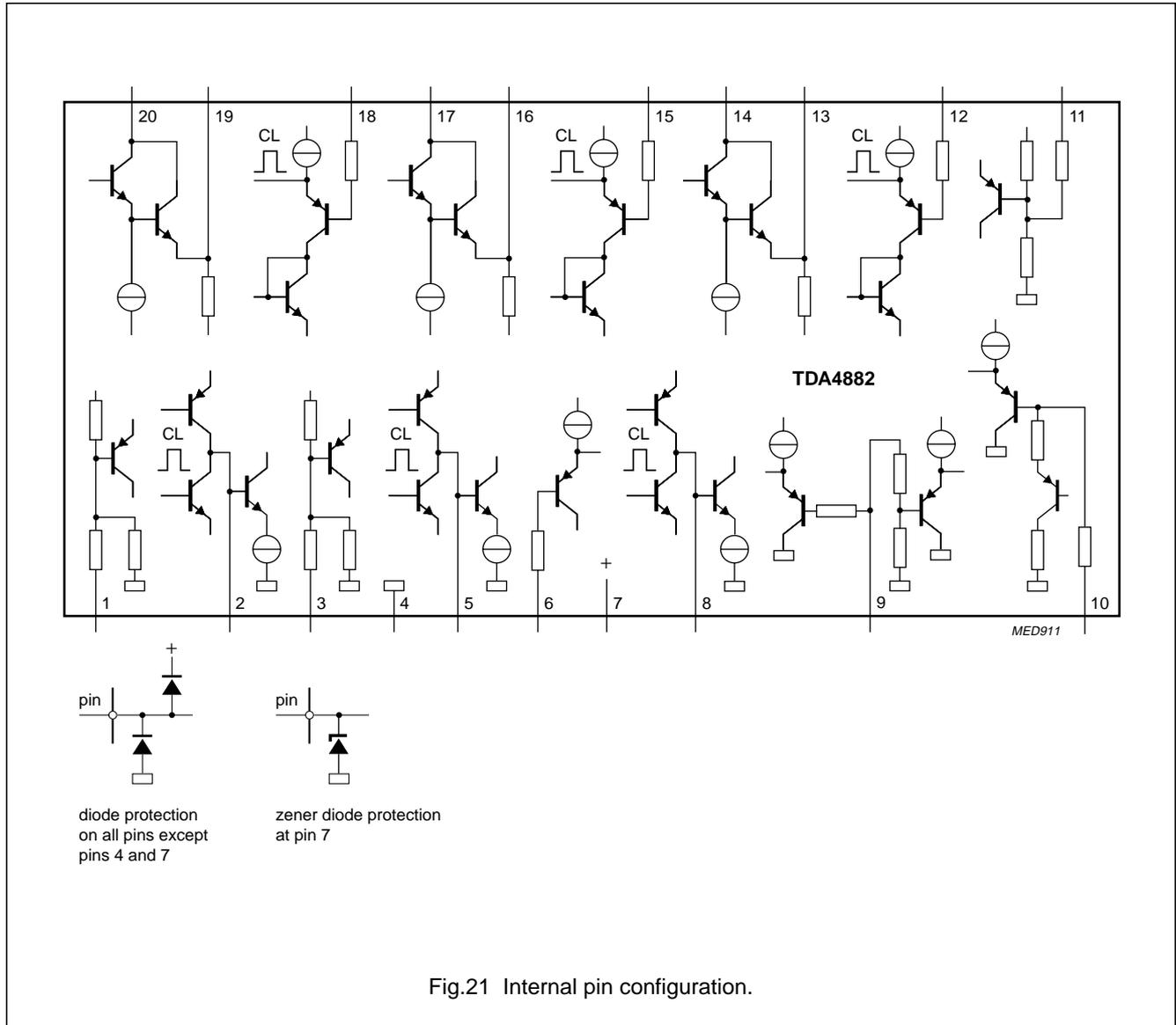
Fig.21 Internal pin configuration.
