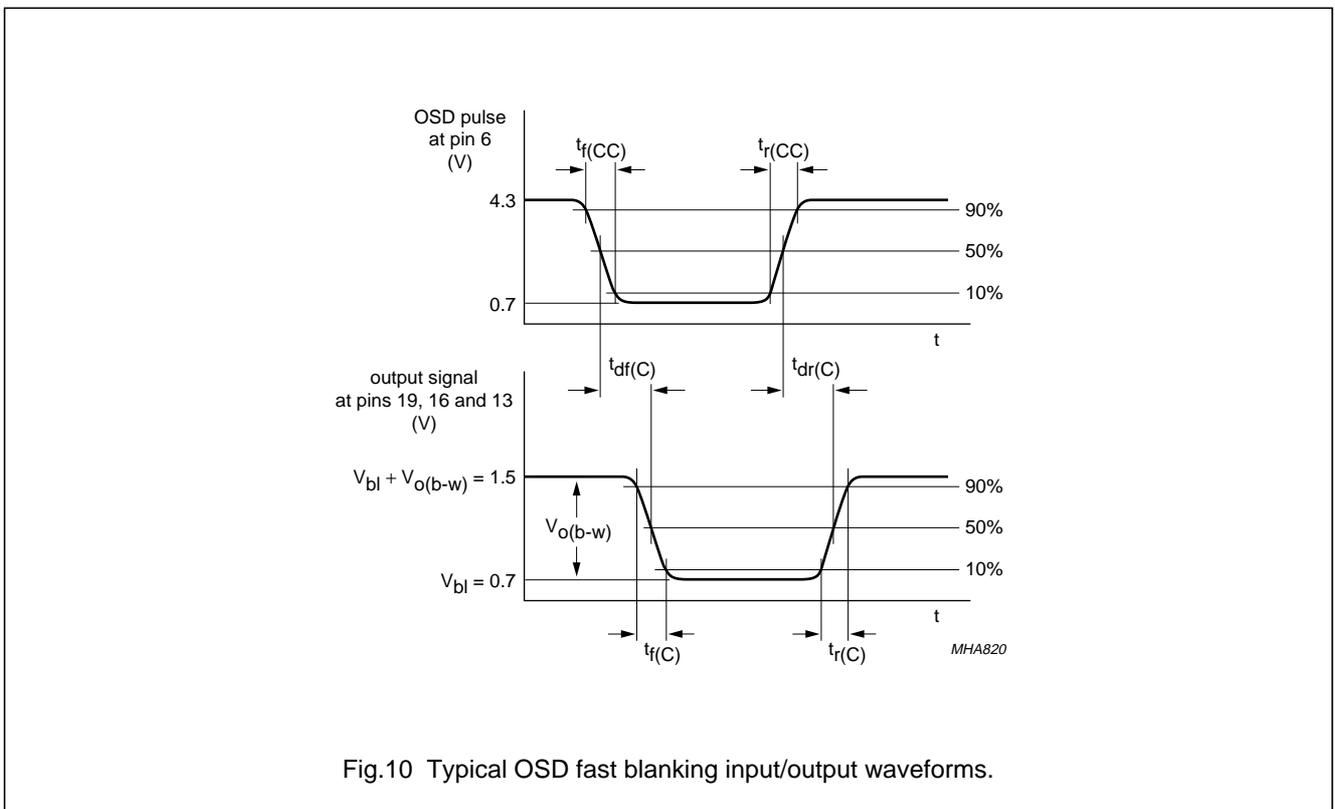
Fig.10 Typical OSD fast blanking input/output waveforms.
