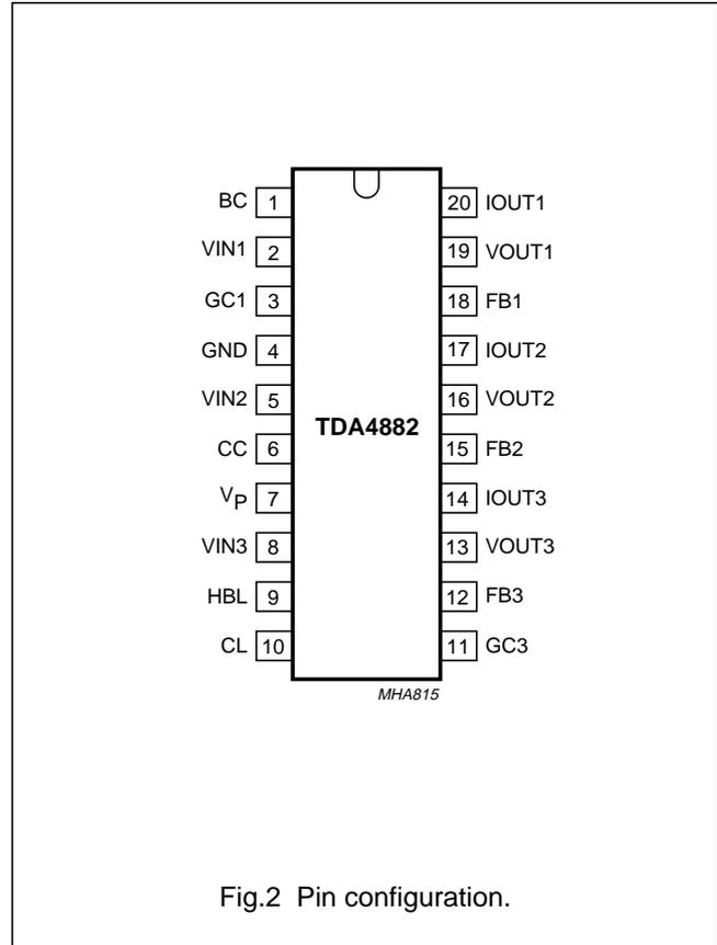
Fig.2 Pin configuration.
