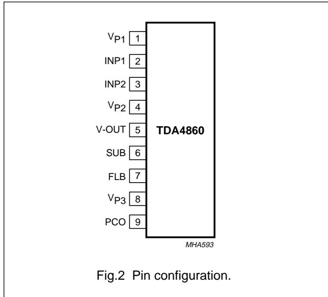
Fig.2 Pin configuration.
