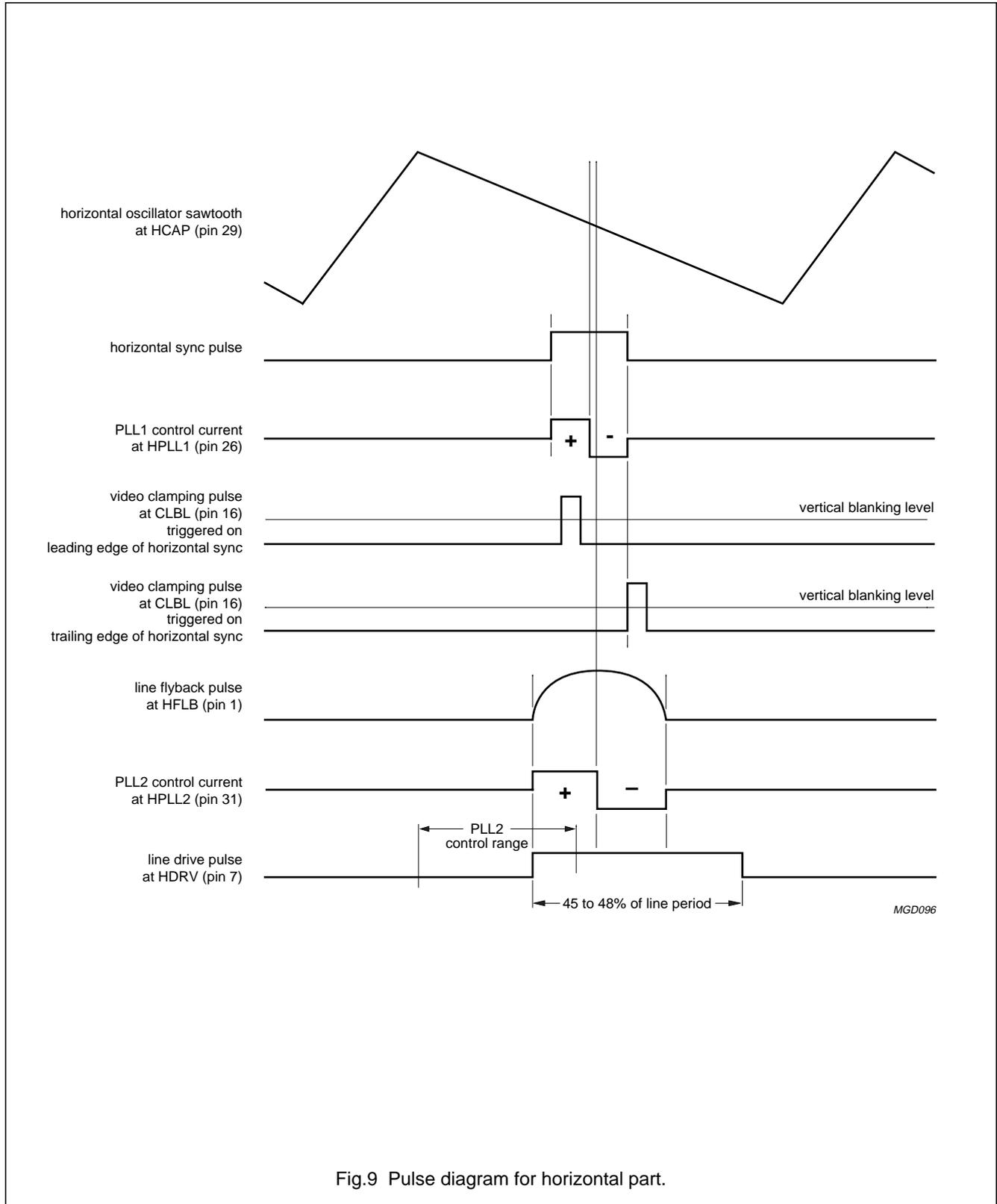
Fig.9 Pulse diagram for horizontal part.
