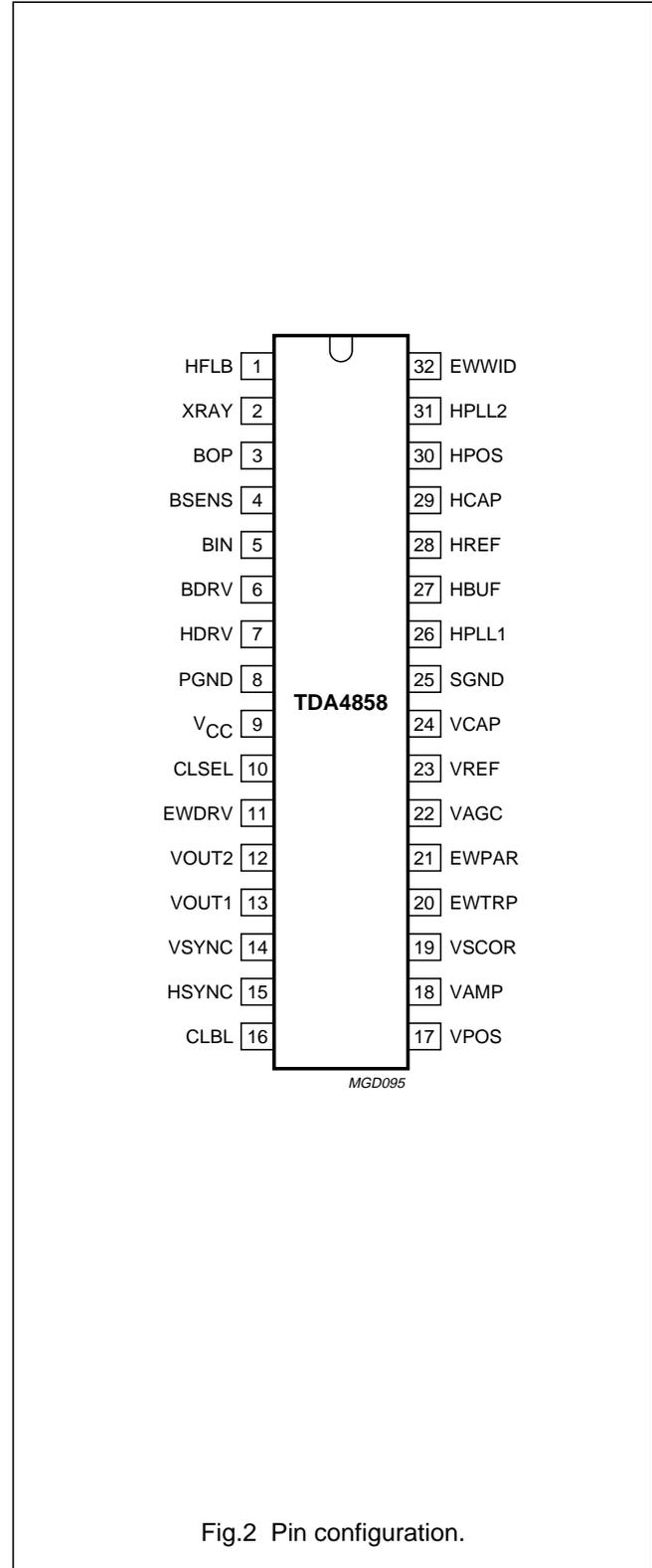
Fig.2 Pin configuration.
