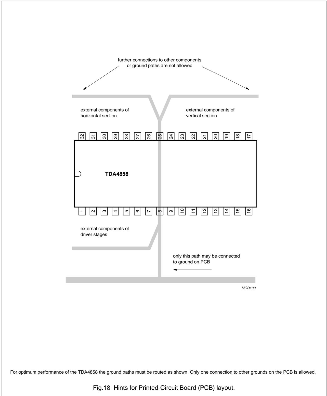
For optimum performance of the TDA4858 the ground paths must be routed as shown. Only one connection to other grounds on the PCB is allowed.
