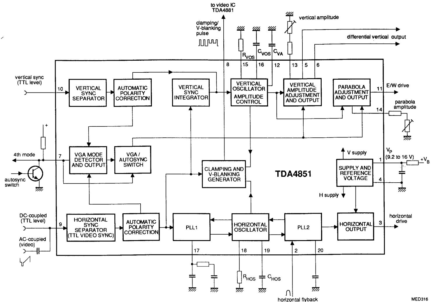
Fig.1 Block diagram.
