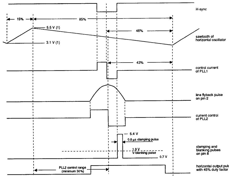
Fig.6 Horizontal timing diagram.
