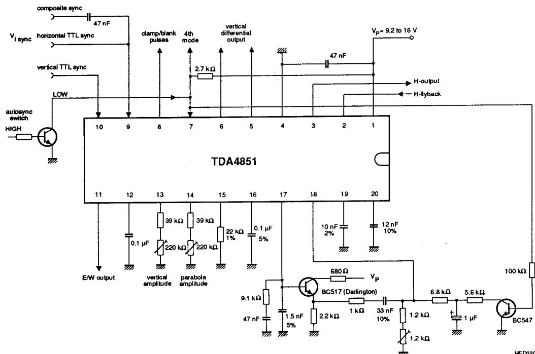
Fig.5 31 to 64 kHz application including 4-mode VGA.
