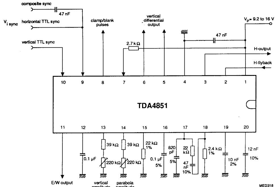
Fig.3 Application circuit for 3-mode VGA (31.45 kHz).
