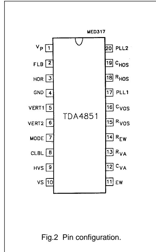
Fig.2 Pin configuration.
