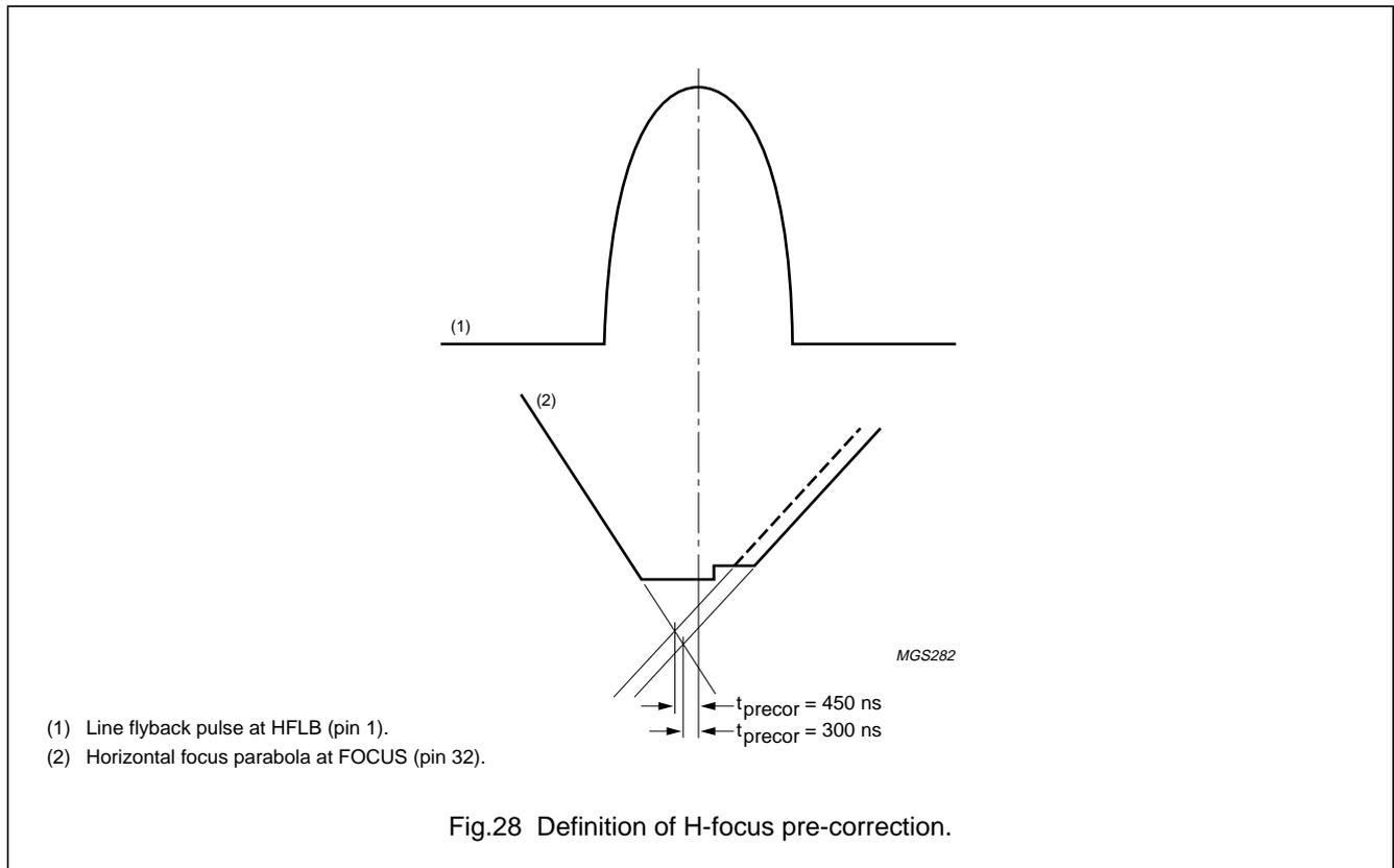
Fig.28 Definition of H-focus pre-correction.
