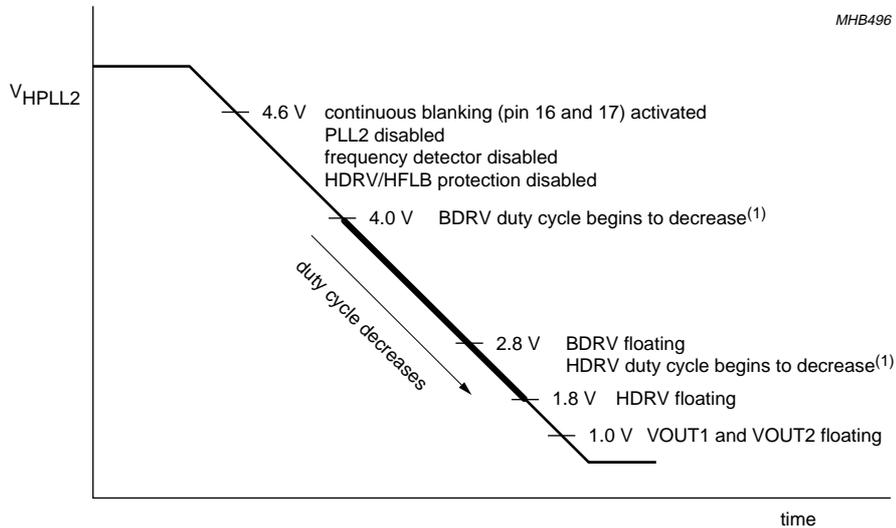
b. Soft-down sequence for  $V_{CC} > 8.6$  V.
