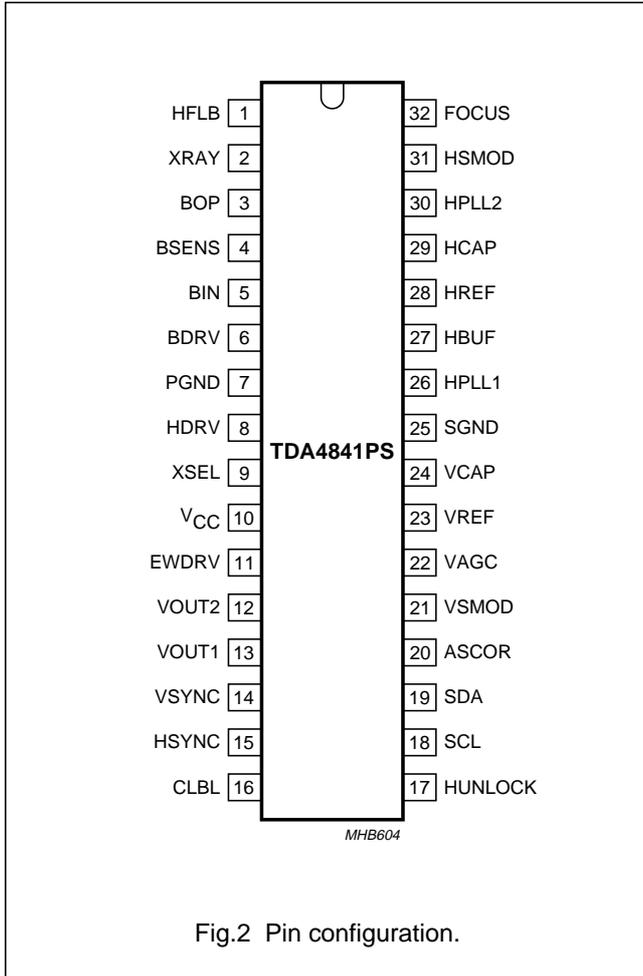
Fig.2 Pin configuration.
