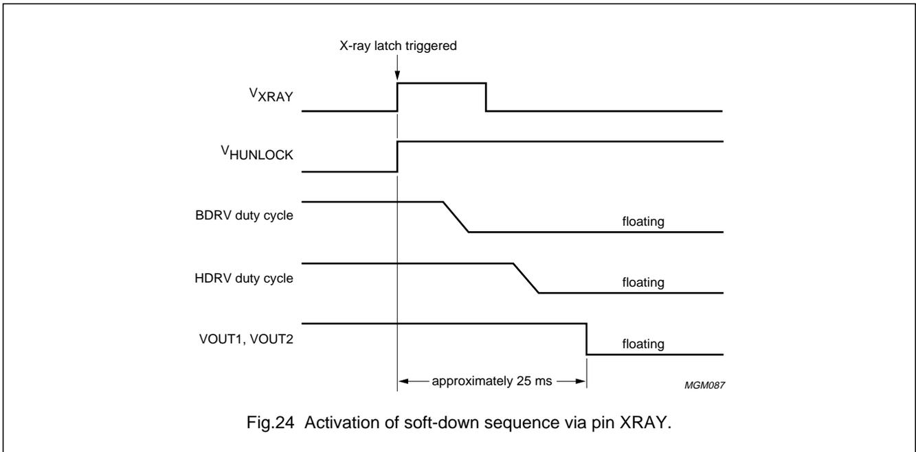
Fig.24 Activation of soft-down sequence via pin XRAY.
