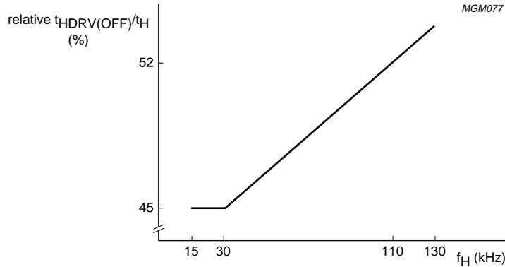
Fig.16 Relative t<sub>OFF</sub> time of HDRV as a function of horizontal frequency.
