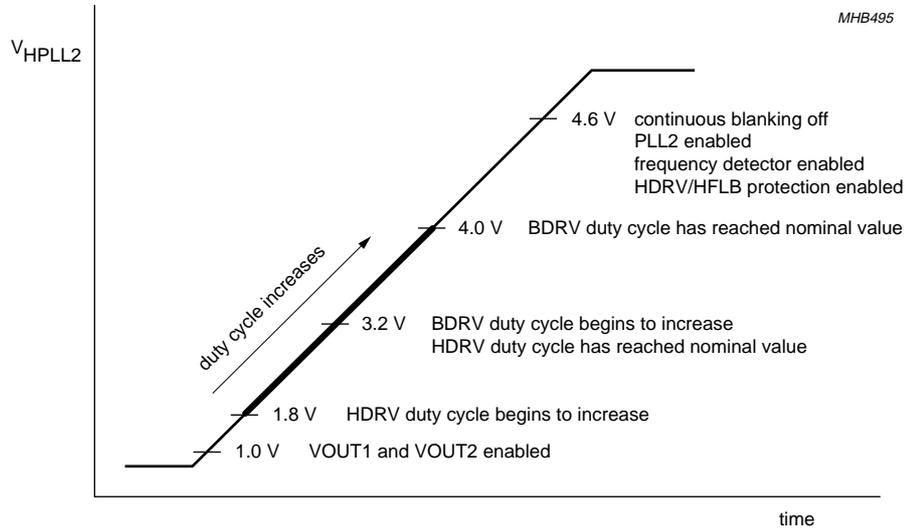
a. Soft-start sequence for  $V_{CC} > 8.6$  V.
