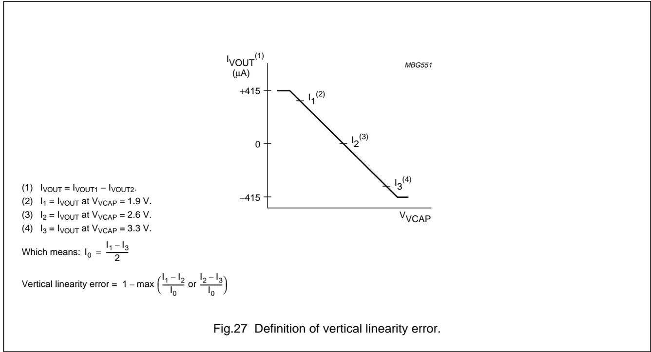
Fig.27 Definition of vertical linearity error.
