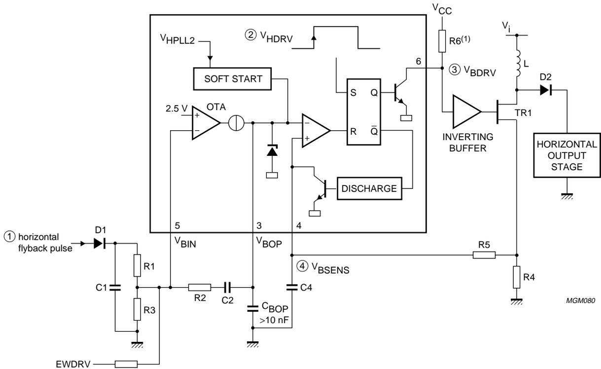
For  $f < 50$  kHz and  $C2 < 47$  nF calculation formulas and behaviour of the OTA are the same as for an OP. An exception is the limited output current at BOP (pin 3). See Chapter "Characteristics", subheading "B+ control section; see Figs 25 and 26".
