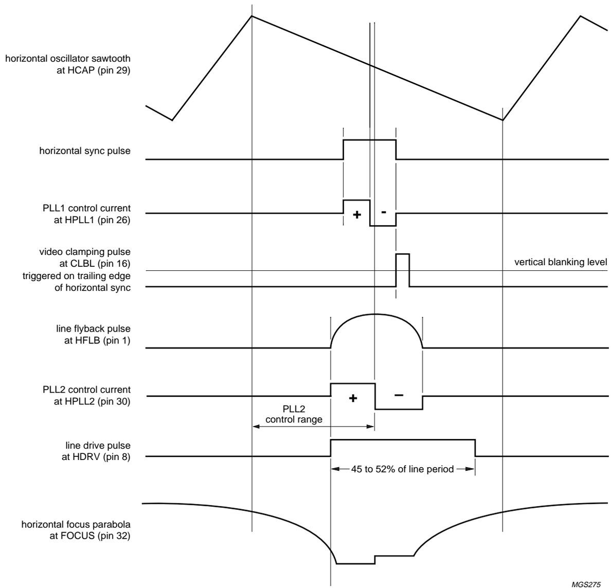
Fig.15 Pulse diagram for horizontal part.
