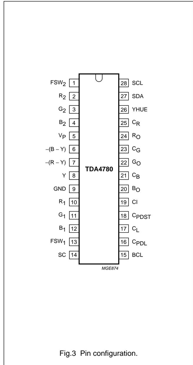
Fig.3 Pin configuration.
