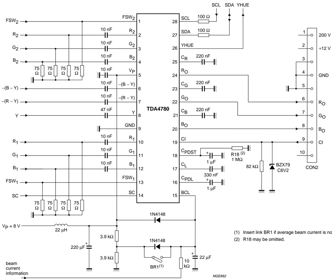
Fig.12 Test and application circuit.
