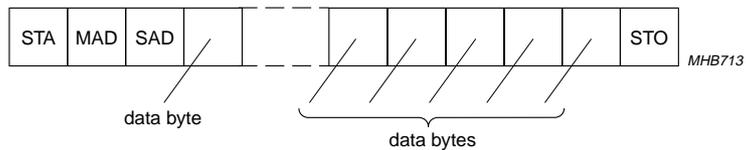
Fig.6 Data transmission with auto-increment (bit BREN = 0).
