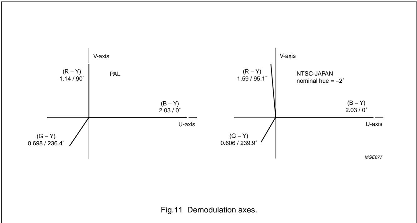
Fig.11 Demodulation axes.
