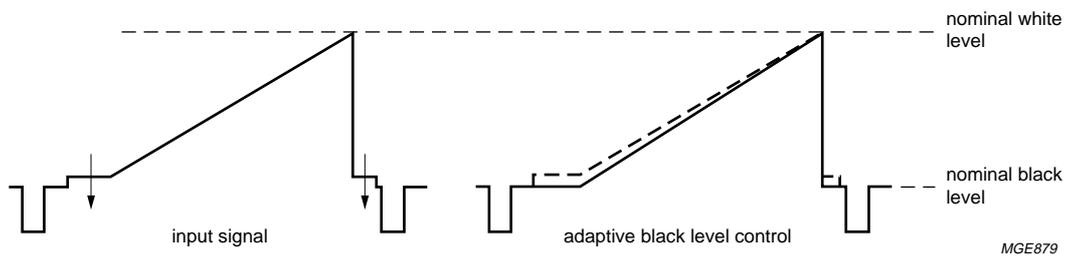
Fig.8 Principle of adaptive black control.
