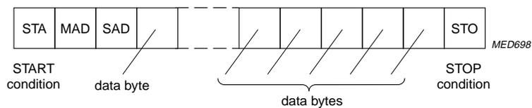
Fig.6 Data transmission with auto-increment (BREN = 0).
