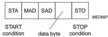
Fig.5 Data transmission without auto-increment (BREN = 0 or 1).
