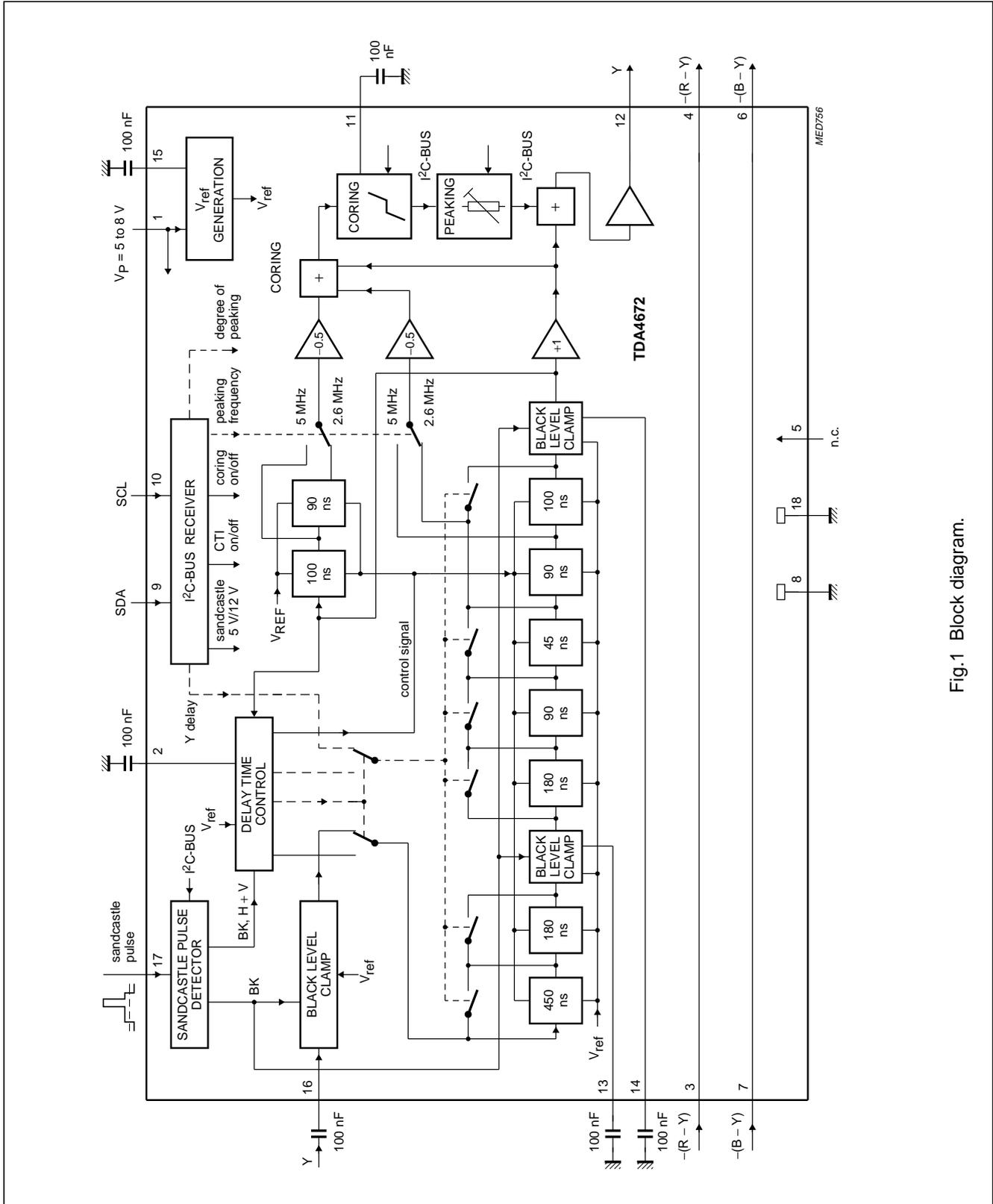
Fig.1 Block diagram.
