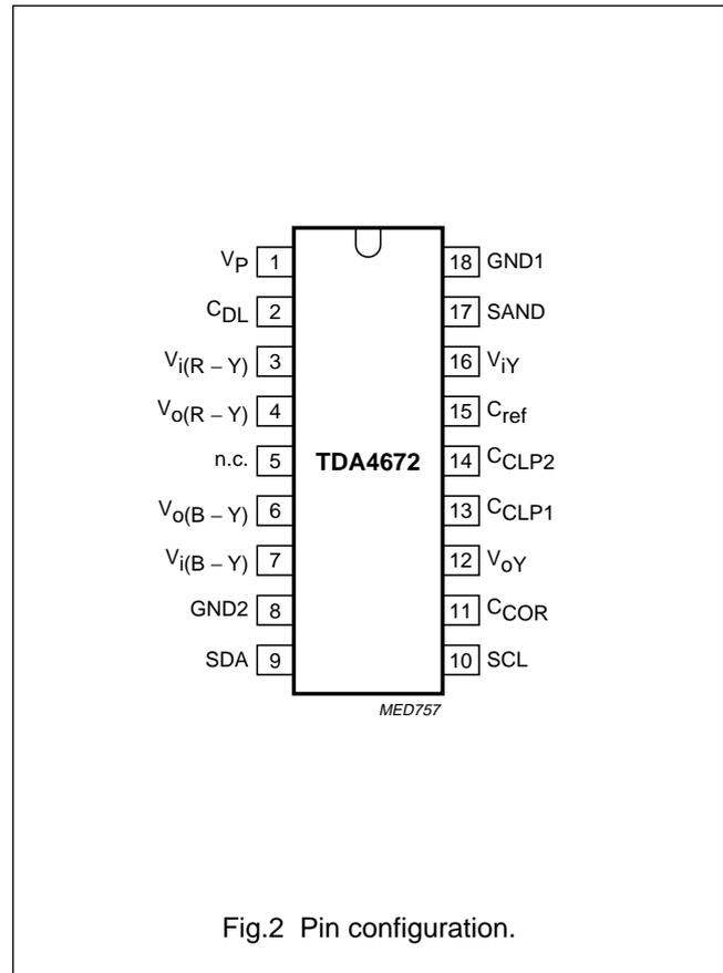
Fig.2 Pin configuration.
