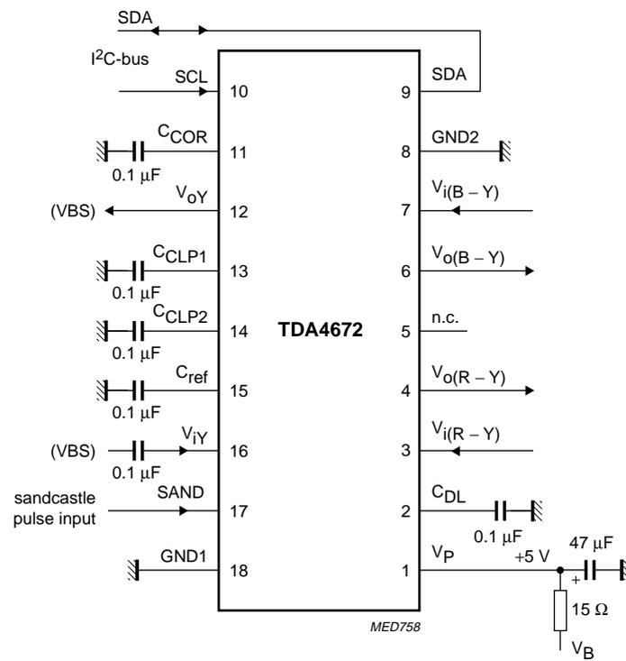
Fig.4 Test and application circuit.
