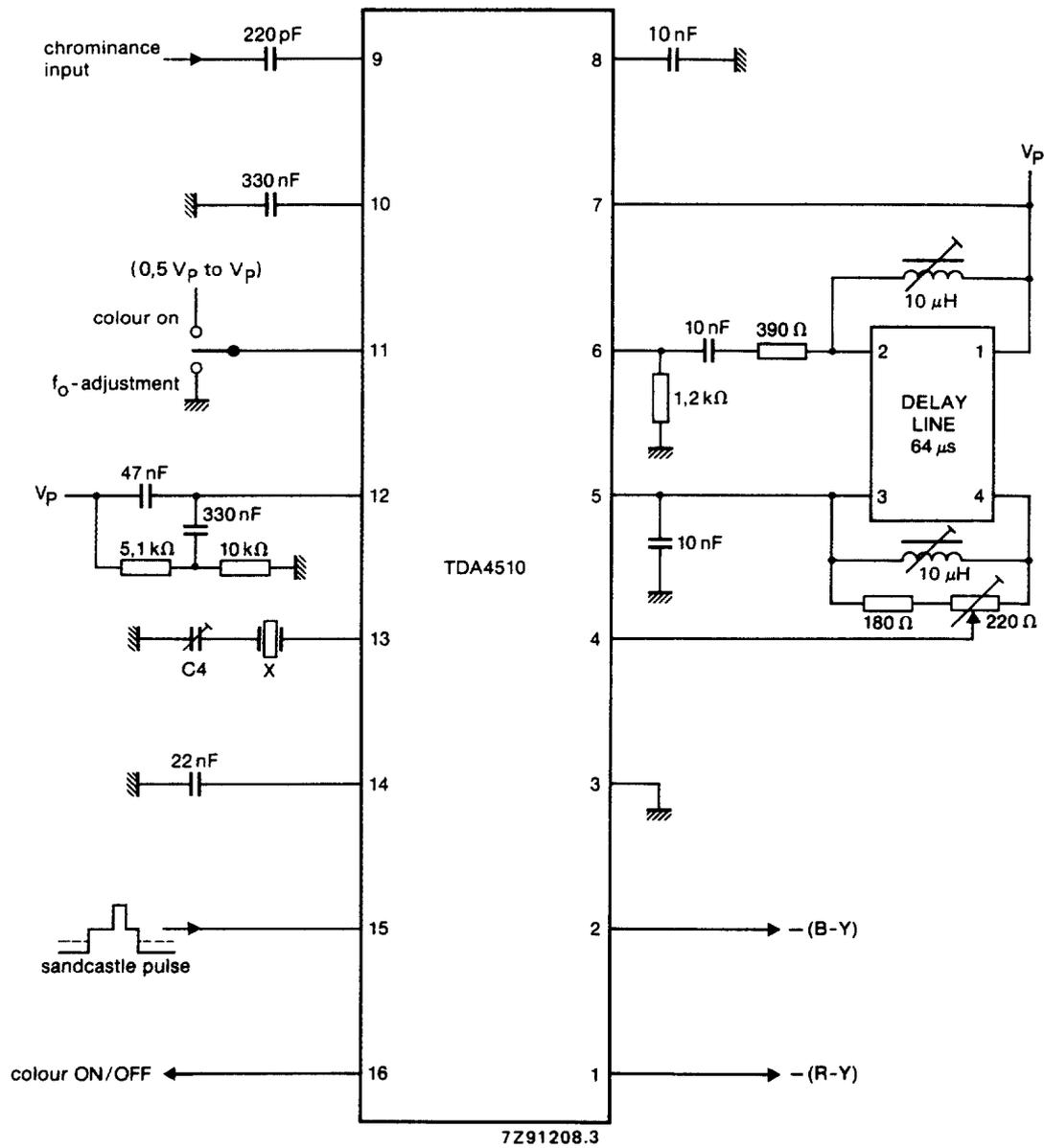
C4 = 5 to 27 pF, X = 8,8 MHz; nominal frequency 8,867 238 MHz; resonance resistance 60 Ω, load capacitance 20 pF, dynamic capacitance 22 fF and static capacitance 5,5 pF.
