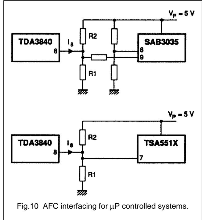
Fig.10 AFC interfacing for  $\mu$ P controlled systems.
