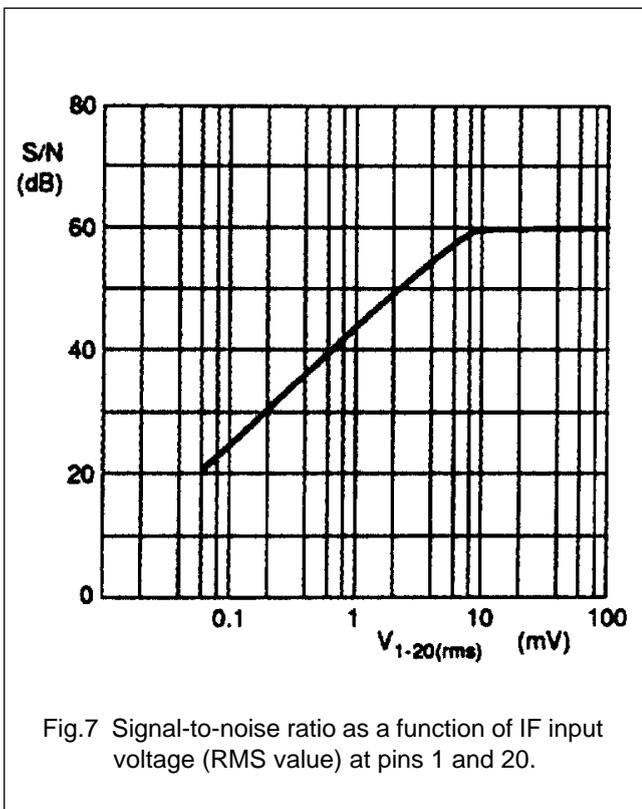
Fig.7 Signal-to-noise ratio as a function of IF input voltage (RMS value) at pins 1 and 20.
