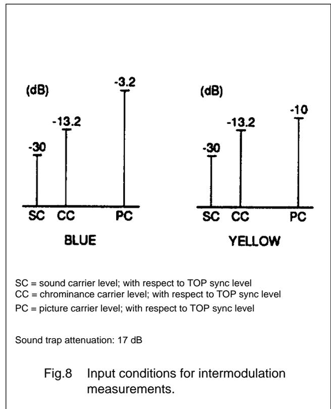
Fig.8 Input conditions for intermodulation measurements.
