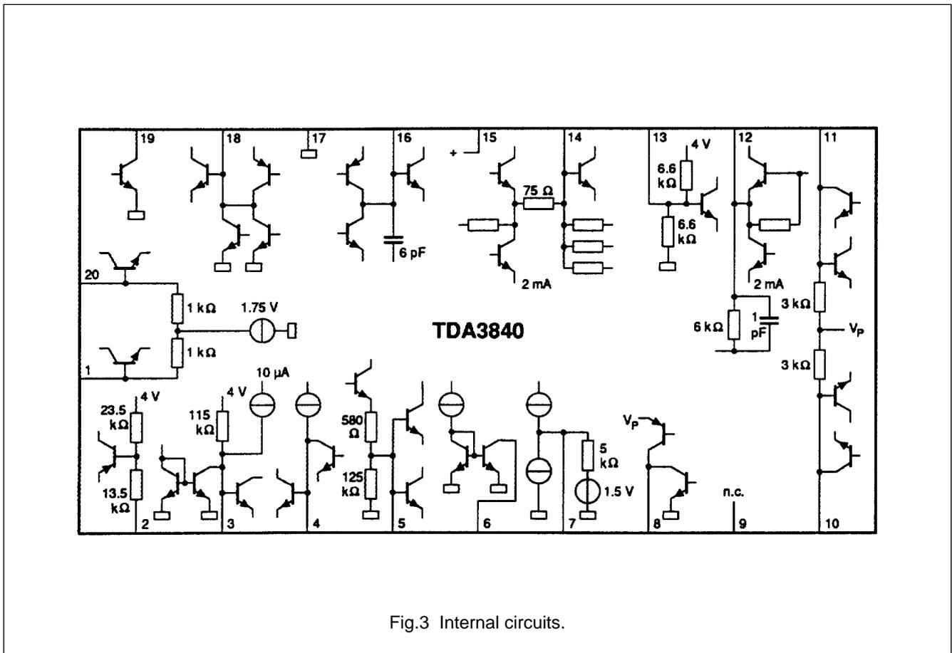
Fig.3 Internal circuits.
