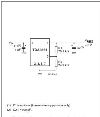
Fig.6 Application circuit with backup function.
