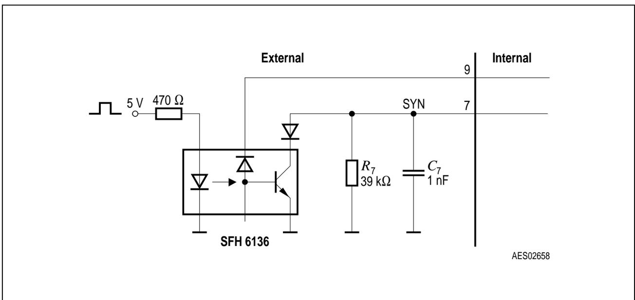
**Figure 13 Ext. Synchronization Circuit**
