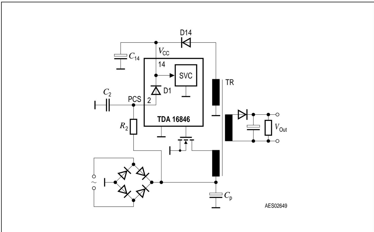
**Figure 4** Startup Circuit
