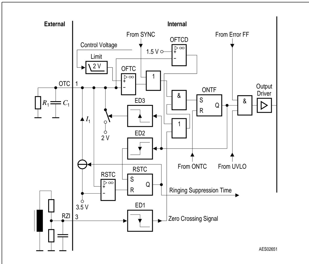
**Figure 6 Off-Time-Circuit**
