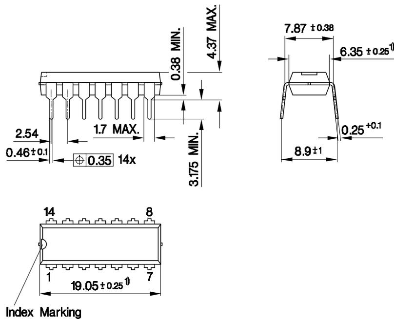
1) Does not include plastic or metal protrusion of 0.25 max. per side
