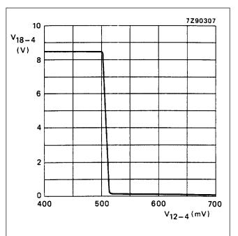
Fig.3 Keyed a.g.c. output voltage  $V_{18-4}$  as a function of input voltage  $V_{12-4}$ . Measured in test circuit Fig.1 at  $V_{3-4} = 2 \text{ V}$ ;  $I_{18} = \phi$ .
