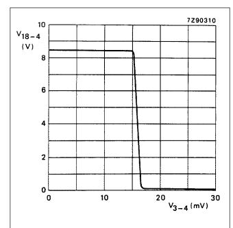
Fig.2 Keyed a.g.c. output voltage  $V_{18-4}$  as a function of r.m.s. input voltage  $V_{3-4}$ . Measured in test circuit Fig.1 at  $V_{12-4} = 0.7 \text{ V}$ ;  $I_{18} = \phi$ .
