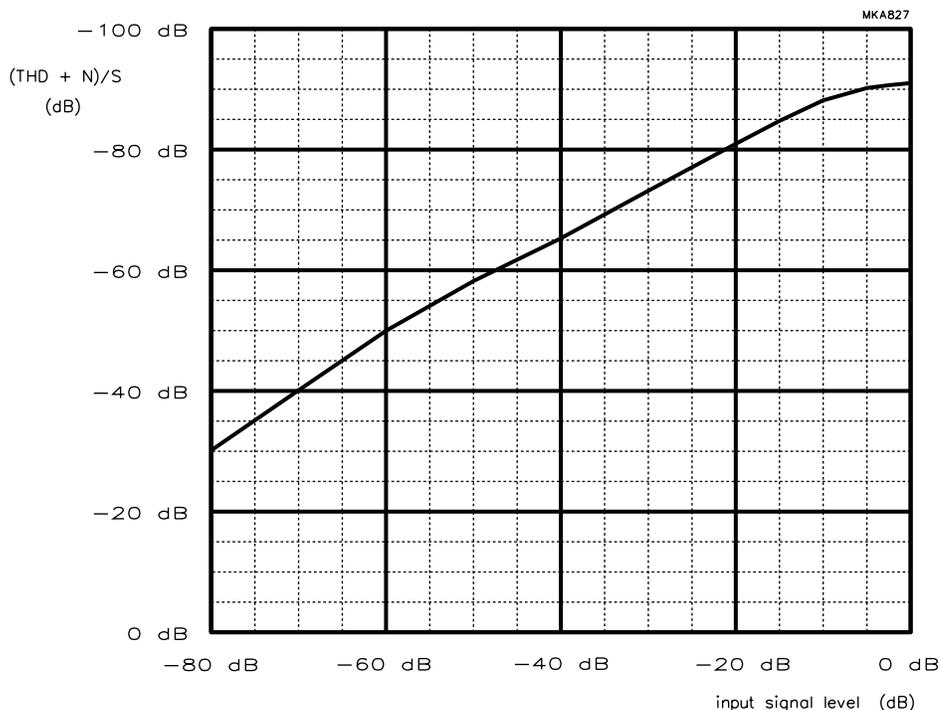
Fig.9 Total harmonic distortion plus noise-to-signal ratio as a function of signal level; (A-weighted).
