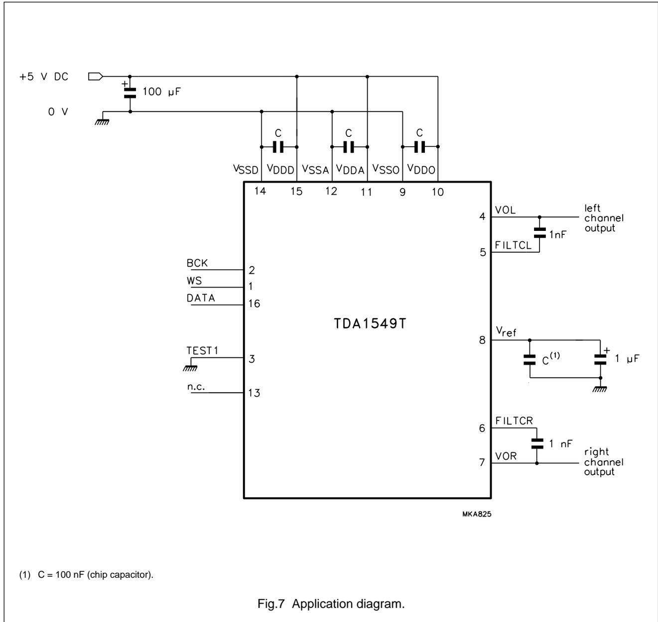
Stereo  $4f_s$  data input up-sampling filter with
