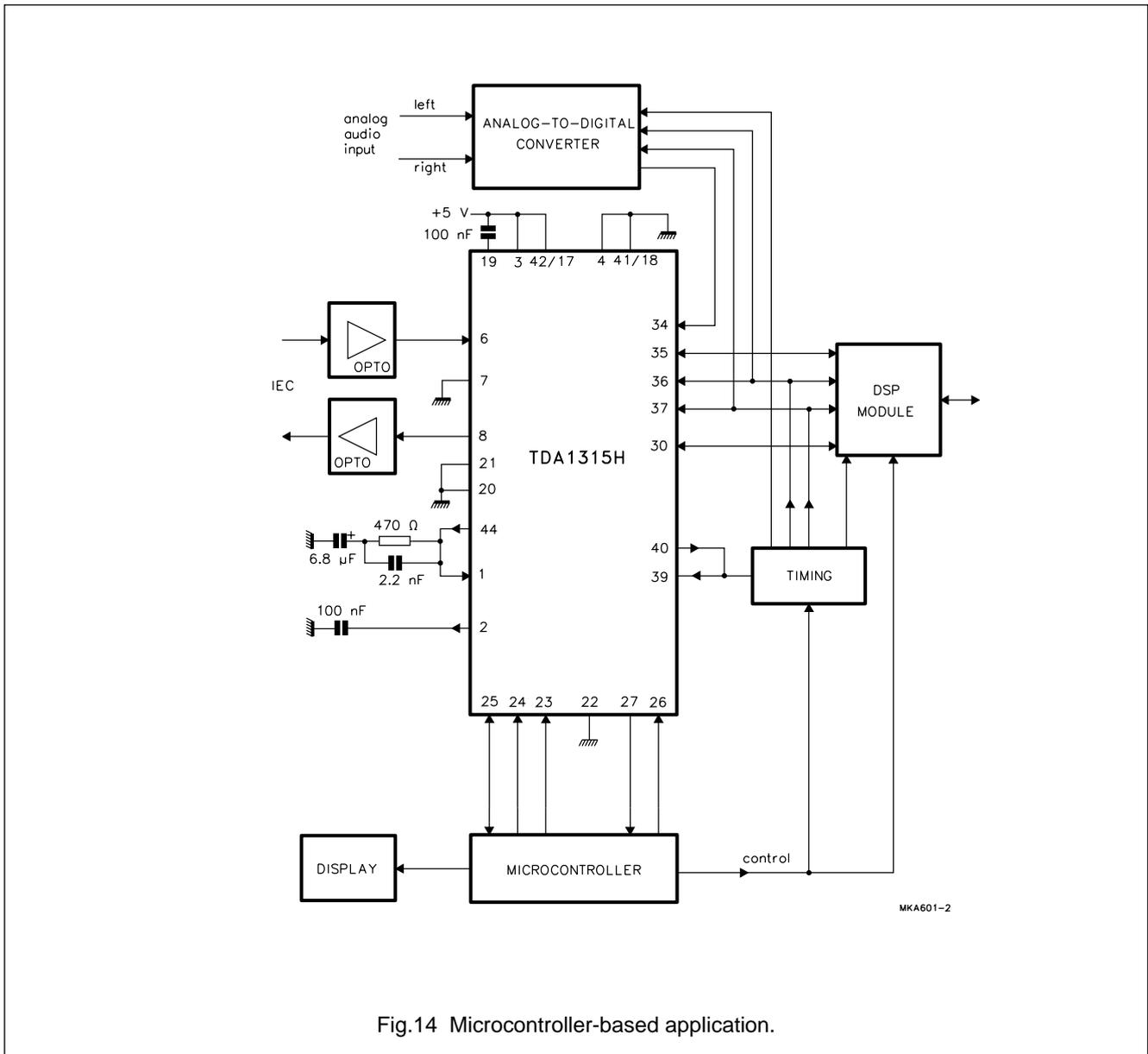
Fig.14 Microcontroller-based application.
