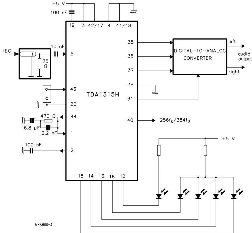
When in a system both IECIN1 and IECIN0 inputs are used, the signal that is applied to the IECIN0 input must be kept away from the IECIN1 input on the printed-circuit board. Steep slopes of the IECIN0 input can be seen by the sensitive adjacent IECIN1 input. An extra capacitance parallel to the 75 Ω resistor, close to the TDA1315H, can help reduce the crosstalk if required. A suitable value is 180 pF.
