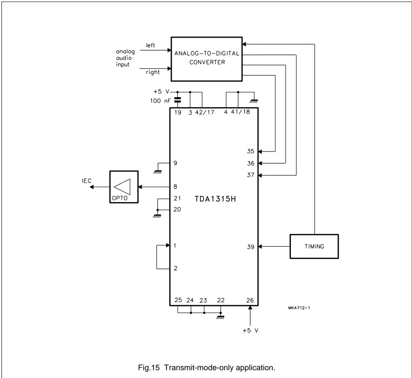
Fig.15 Transmit-mode-only application.
