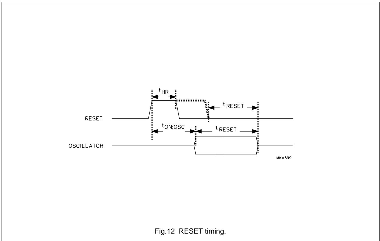
Fig.12 RESET timing.
