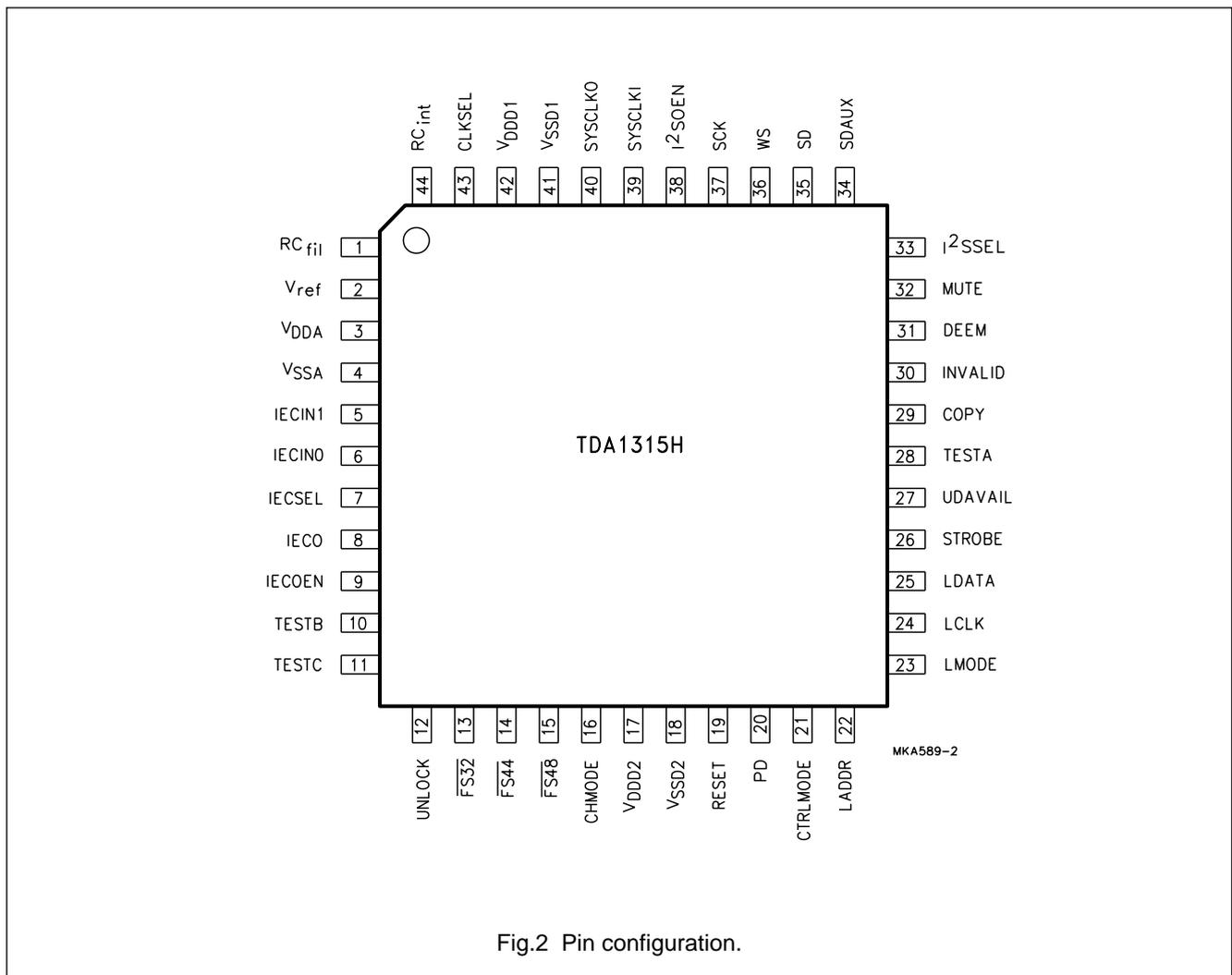
Fig.2 Pin configuration.
