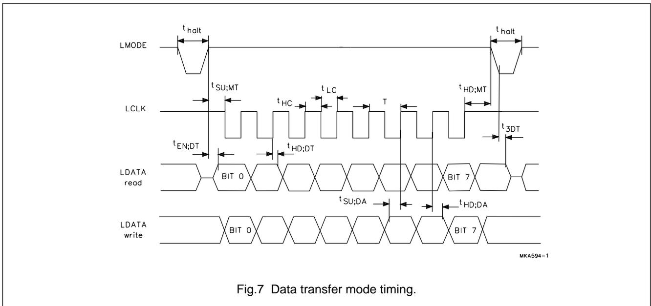
Fig.7 Data transfer mode timing.
