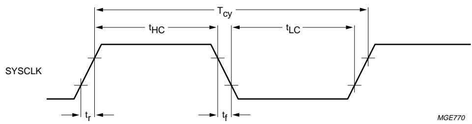
Fig.7 Serial timing of SYSCLK related signals.
