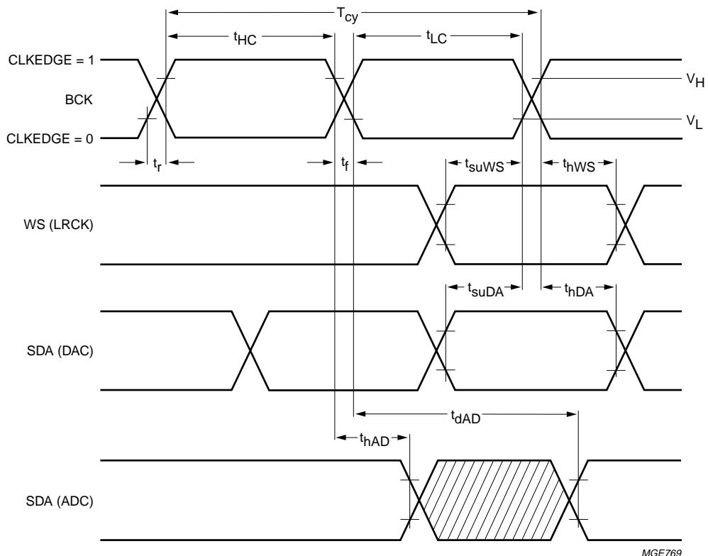
Fig.6 Serial timing of BCK related signals.
