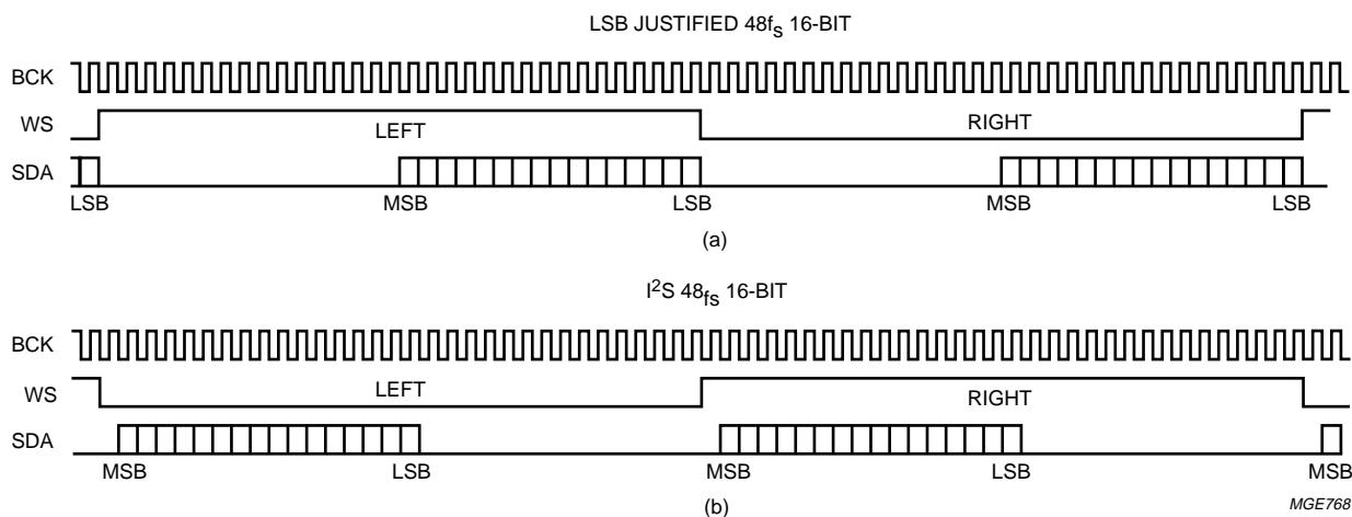
Fig.4 DAC and ADC data formats (continued from Fig.3).
