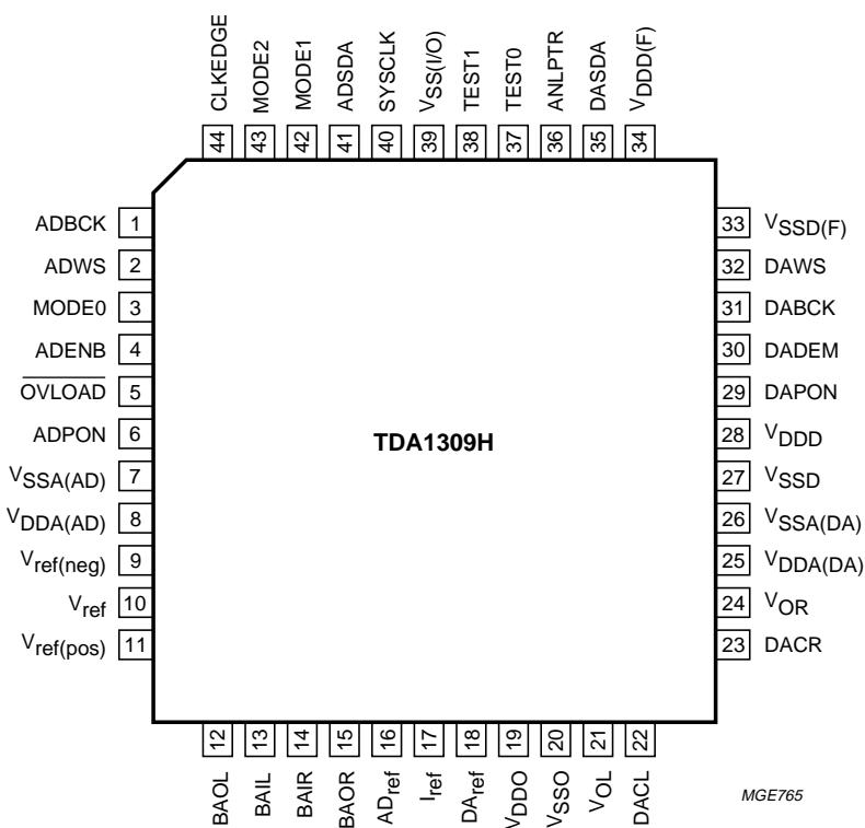
Fig.2 Pin configuration.
