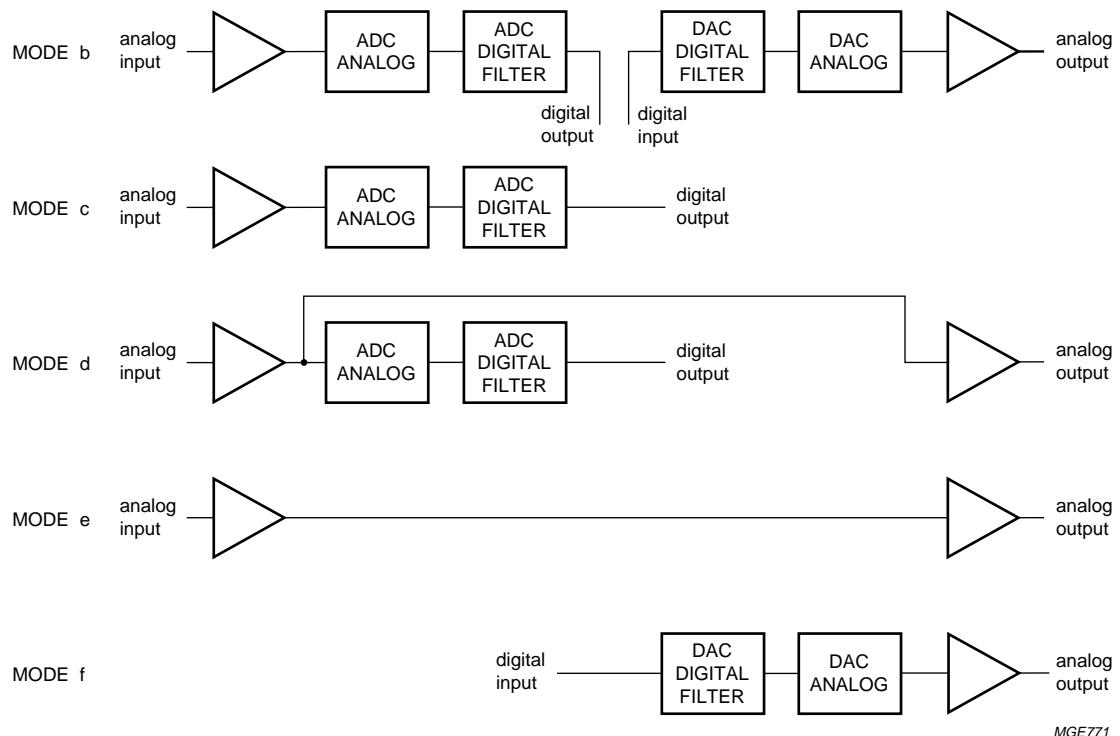
Fig.5 Schematic diagram of operating modes.
