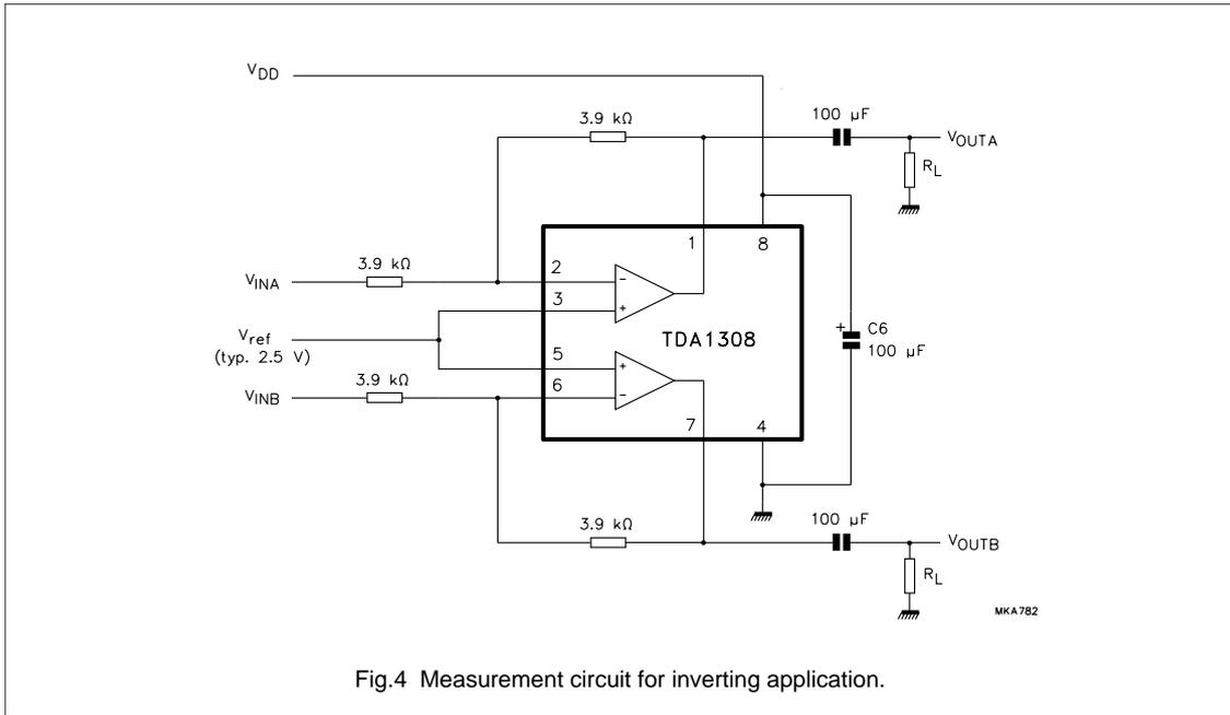
Fig.4 Measurement circuit for inverting application.
