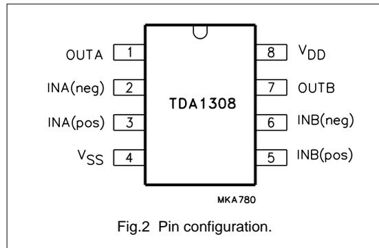
Fig.2 Pin configuration.
