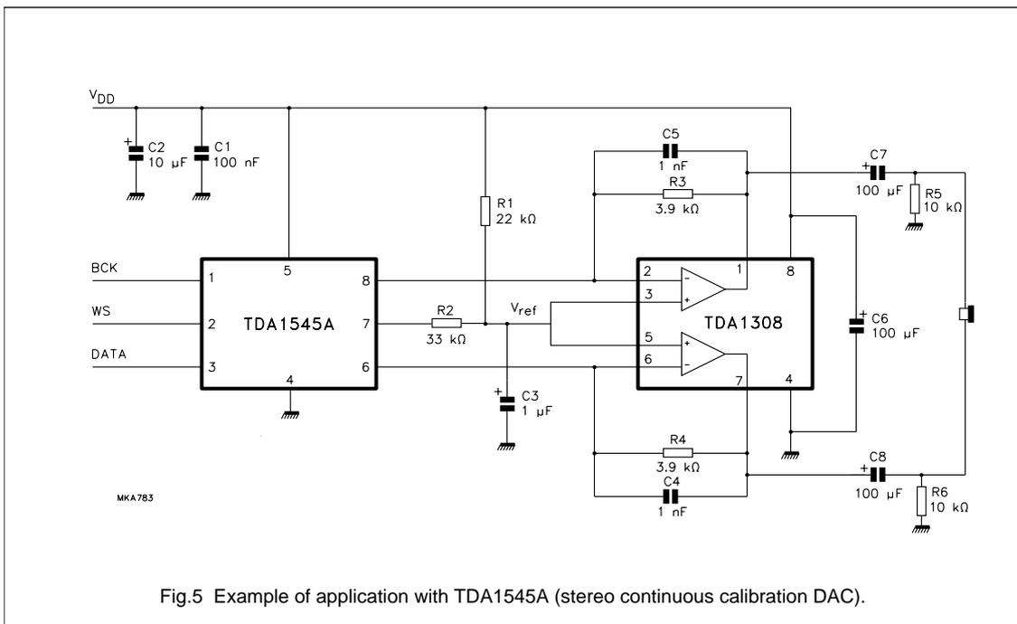
Fig.5 Example of application with TDA1545A (stereo continuous calibration DAC).
