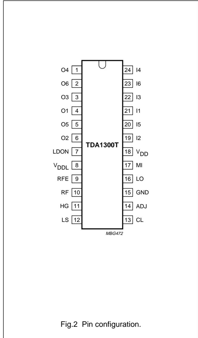
Fig.2 Pin configuration.
