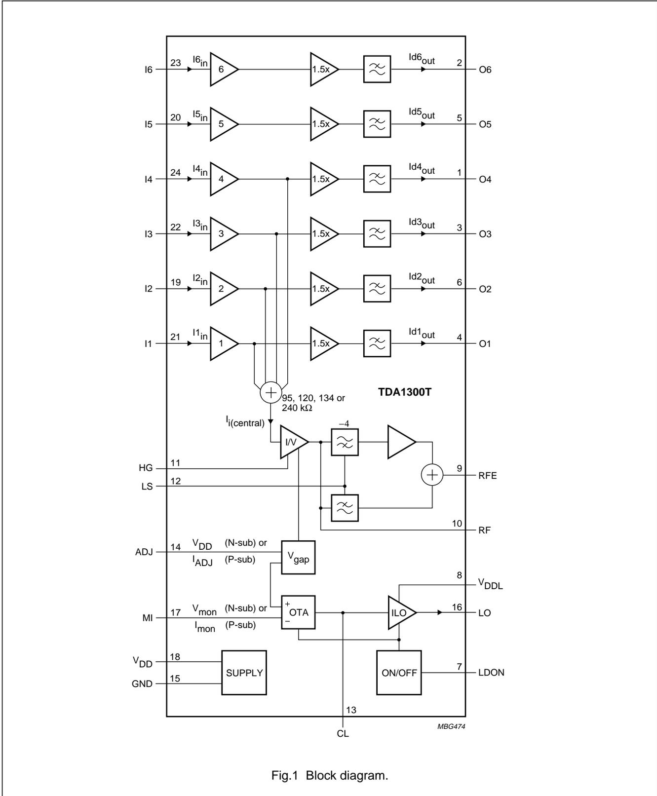
Fig.1 Block diagram.
