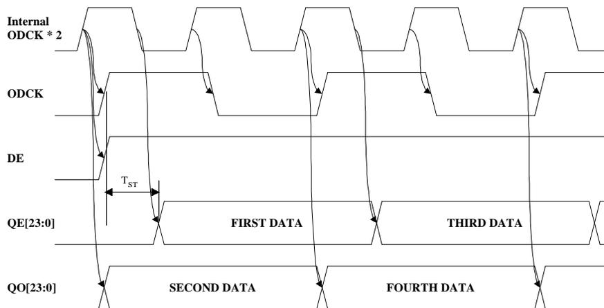
Figure 7. TFT 2-Pixels/Clock Staggered Output Timing Diagram
