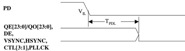
Figure 5. Output Signals Disabled Timing from PD Active
