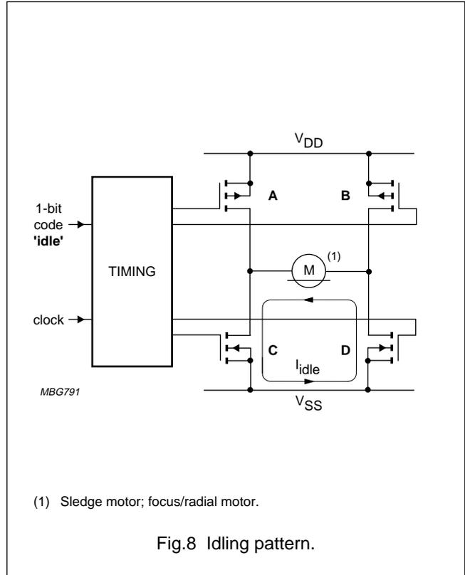
(1) Sledge motor; focus/radial motor.
