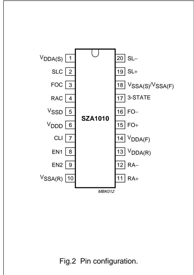
Fig.2 Pin configuration.
