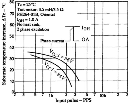
Fig. 26  $\tau - \text{Input pulse}$  characteristics
