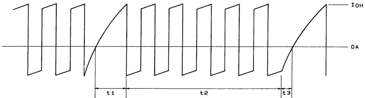
**Fig. 16 Motor Output Current Waveform (idealized model)**
