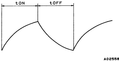
Fig. 12 R/C Waveform
